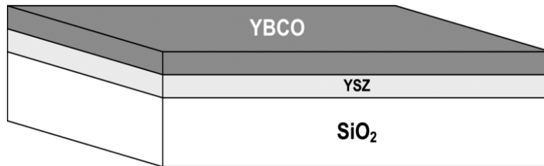
Figure 2.7 The schematic of a superconducting optical waveguide[45], Reprinted from Ieee Transactions on Applied Superconductivity, 18(4), B.G. Ghamsari, Theory of superconductive traveling-Wave photodetectors, 1761-1768, Copyright(2008), , with permission from Copyright Clearance Center, All rights reserved.
