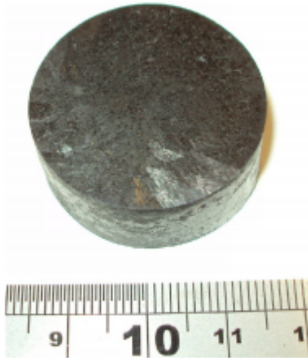
Figure 2.8 Photograph of a large Y-123 single crystal (30 mm diameter and 12 mm height) [53], Reprinted from Superconductor Science & Technology, 35(7), Babu, N.H., Growth of large sized \text{YBa}_2\text{Cu}_3\text{O}_7 single crystals using the top seeded melt growth process, Copyright(2012), with permission of IOP Publishing. All rights reserved.
