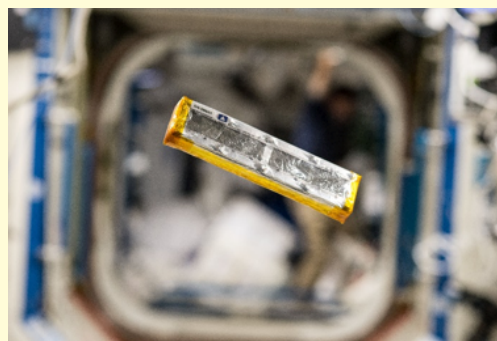
The Synthetic Muscle Experiment: Shown here is one of four aluminum protective cages housing eight synthetic muscle samples on the ISS-NL. Source: NASA, photographer Astronaut Scott Kelly
