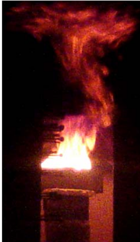
Figure 4-7: Picture of the sustained external burning with the burner at h/H_{\text{Door}} = 75\% and an ideal heat release rate of 52 kW
