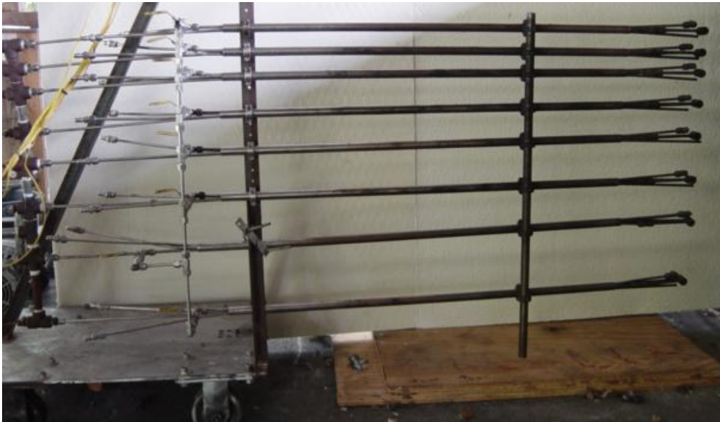
Figure 2-14: Picture of the compartment door sampling rake.
