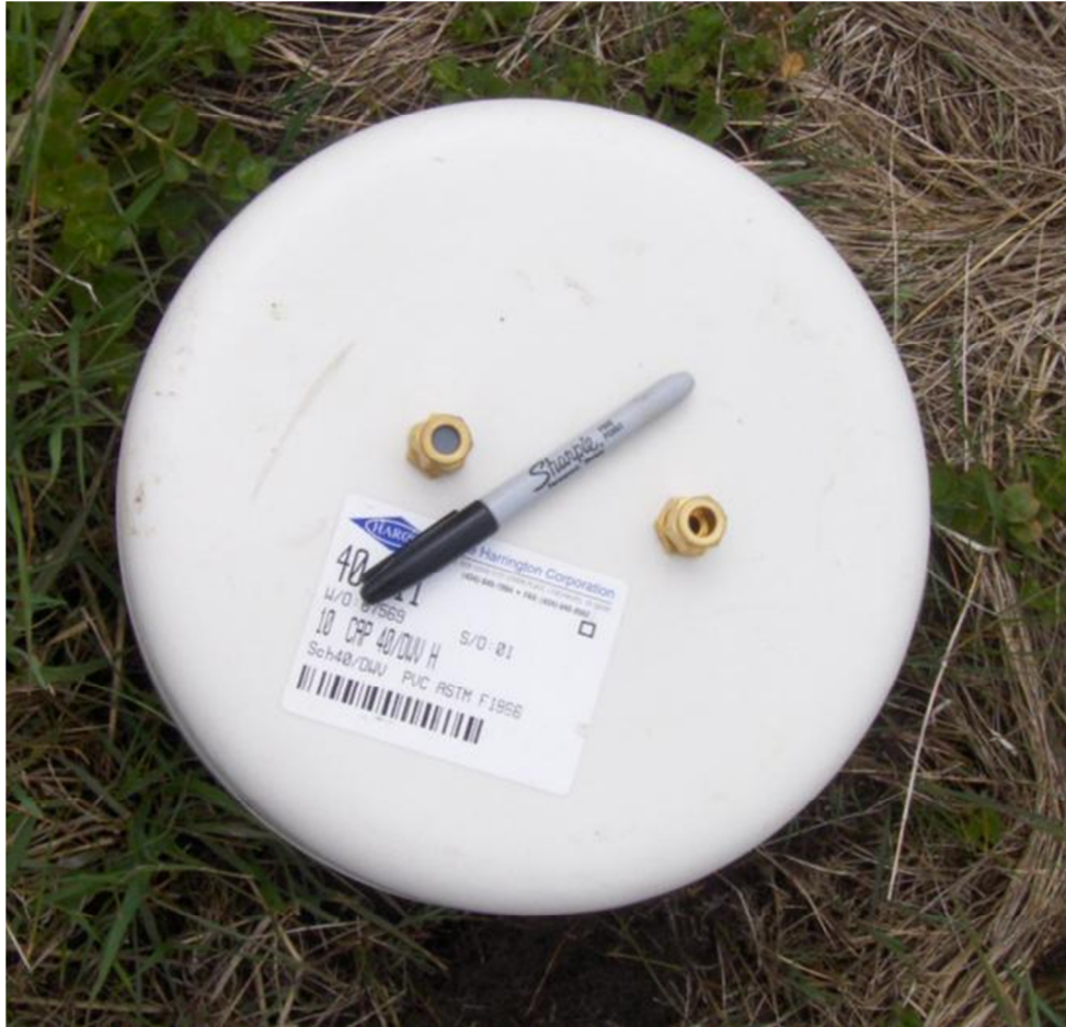
Figure A-2: Overhead view of mesocosm cap. Sampling port to left with visible grey septum, vent tube port to right. Sharpie® in image for scale.
