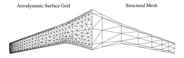
Figure 4.1: Discretization for aerodynamic and structural wing models.
