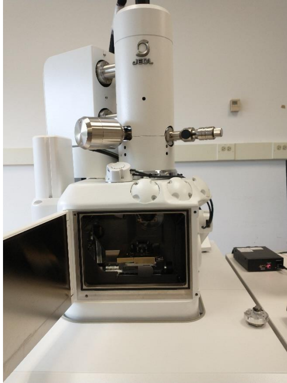
Figure 3-7: JEOL IT500 Scanning Electron Microscope Chamber
