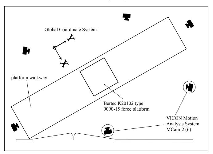
Center of pressure data was collected by Bertec K20102 type 9090-15 force platform and marker position data was collected with the VICON 460 Motion Monitoring System as seen in the configuration above.
