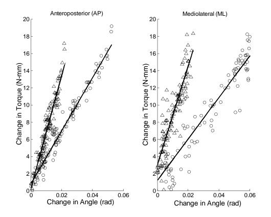
**Figure 3**: Sample data used to calculate unfatigued and fatigued feedforward stiffness values ( $\bigcirc$  – unfatigued values,  $\triangle$  – fatigued values). As can be seen, the data generally had a linear trend which accommodated a linear least-squares fit. Both AP and ML directions demonstrated significant increases in stiffness following lumbar extensor fatigue.
