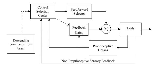
**Figure 2**: Control flow diagram similar to that found in Kuo (1995). The CNS Control Selection Center receives afferent sensory signals from the body. Upon processing this information, two feedforward strategies of balance control, which are not exclusive, are employed during quiet stance. A change in feedforward stiffness and/or a reweighing of sensory information is engaged in feedback control.
