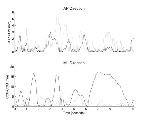
**Figure 4**: Absolute value of unfatigued and fatigued COP-COM signal in AP and ML directions for first ten seconds of a participant. Unfatigued and fatigued values are overlaid for comparison. Notice the increase in fatigued COP-COM amplitude in the AP direction with a simultaneous decrease in fatigued COP-COM amplitude in the ML direction.
