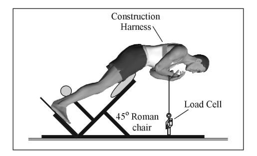
**Figure 1**: Method used to measure isometric MVEs of the lumbar extensors. In this position, participants were instructed to extend at the back as hard as possible.
