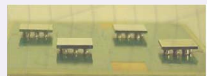
Hour-Glass Shaped Solder Joints
