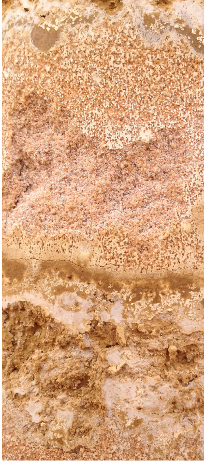
Silt Mixed with Sand Sample Before and After Drying. Silt Mixed with Sand Sample Texture.
