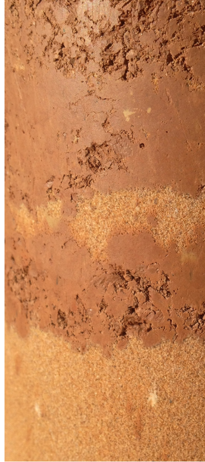
Rocky Soil Mixed with Sand Sample Before and After Drying. Rocky Soil Mixed with Sand Sample Texture.
