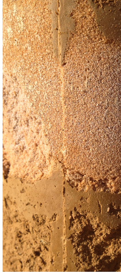
Silt Mixed with Sand Sample Before and After Drying. Silt Mixed with Sand Sample Texture.
