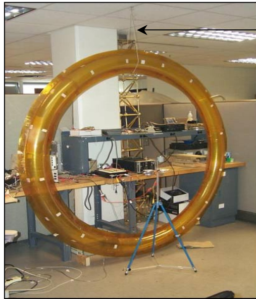
Fig. 4.16: The inflated torus used in experiment (Park, Ruggiero, and Inman, 2002)
