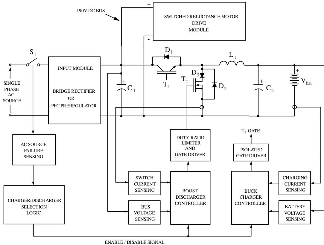
Figure 4.8 The simplified block diagram of the proposed UMD system.
