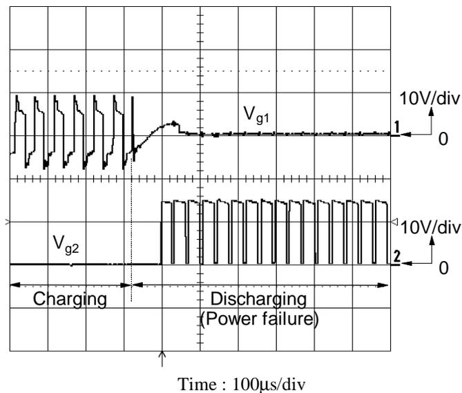
Figure 4.14 Transient gate drive signals for charger/discharger.
