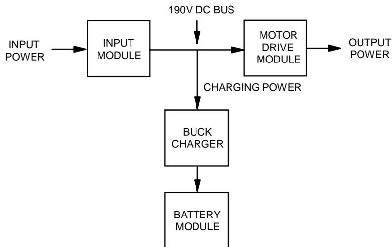
Figure 4.17(i) Power flow in charging mode.
