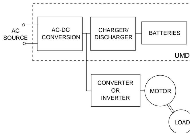
Figure 4.2 The proposed UMD system for VSD.
