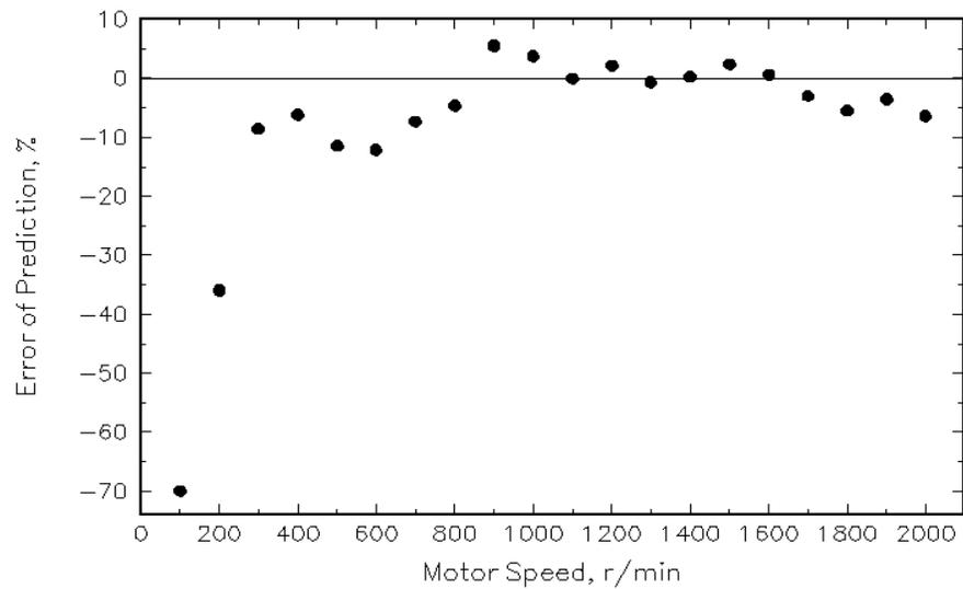
Figure 4.19(v) Prediction error versus SRM speed for UMD overall system efficiency in discharging mode.
