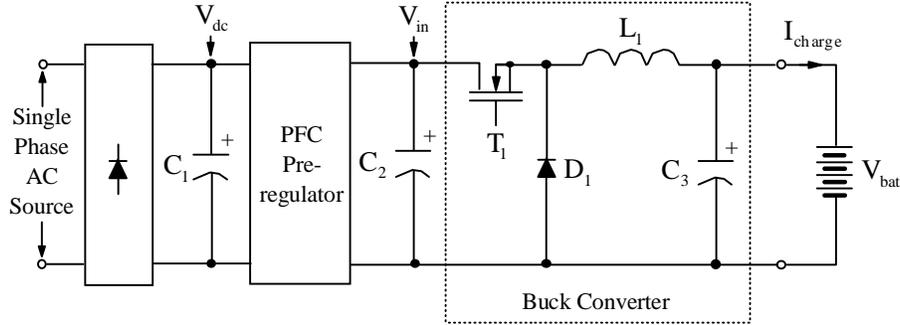
Figure 4.4 Diode bridge rectifier with a PFC preregulator and a buck converter.
