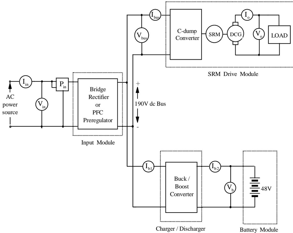
Figure 4.13 Experimental test setup for UMD system with SRM-based VSD.
