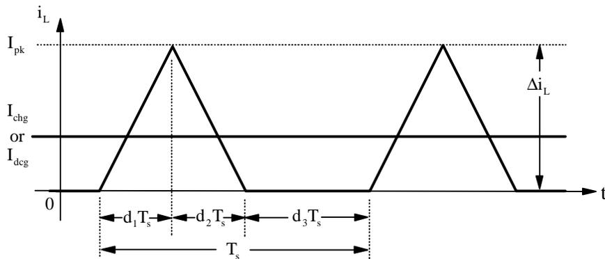
Figure 4.11 Illustration of duty cycles in the proposed charger/discharger.
