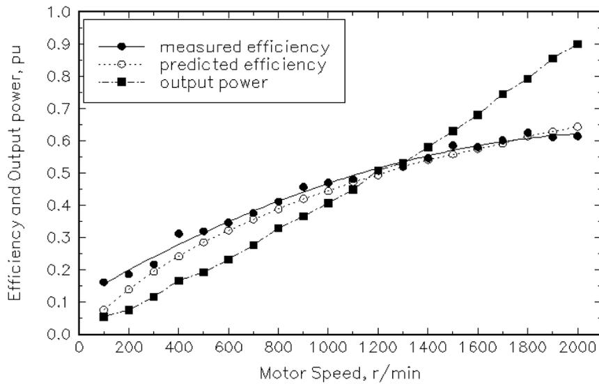
Figure 4.17(iii) Overall system efficiency and normalized output power in charging mode with PFC preregulator.
