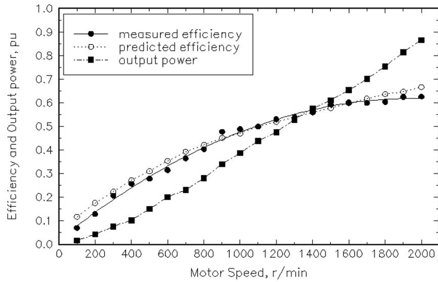
Figure 4.19(iv) Overall system efficiency and normalized output power in discharging mode without PFC preregulator.
