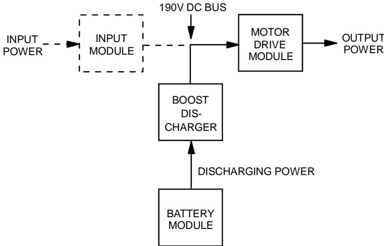
Figure 4.19(i) Power flow in discharging mode.
