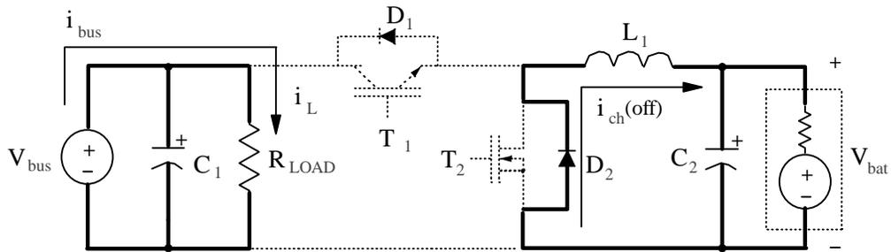
Mode II:  $T_1$  and  $T_2$  off (charging mode)
