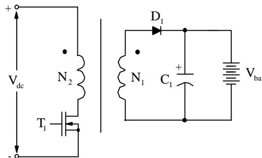
Figure 4.5 Charger with high frequency transformer isolation.
