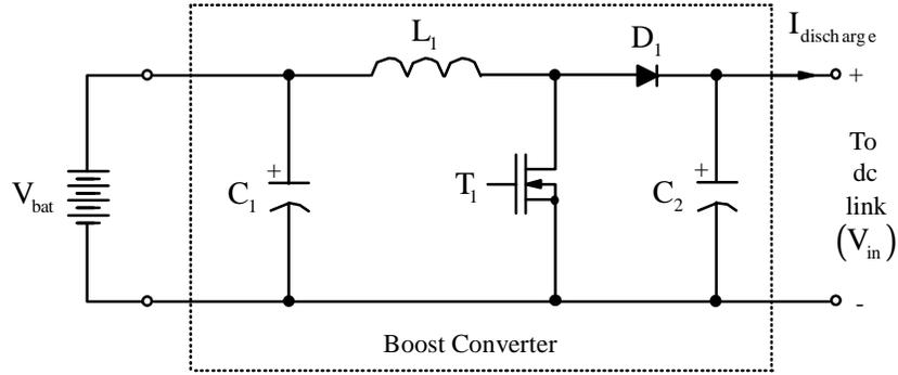
Figure 4.6 Boost converter as a discharger.
