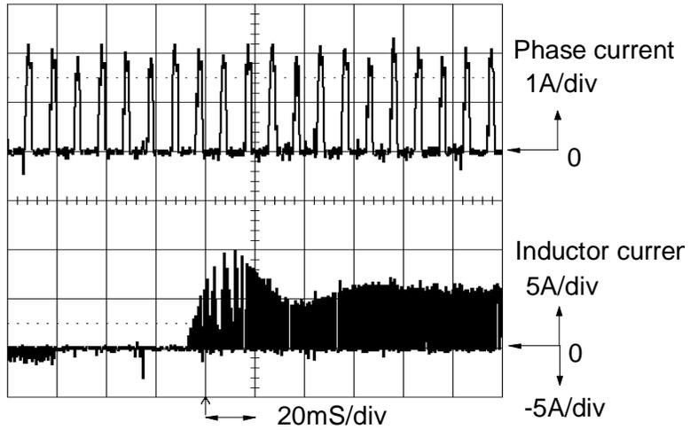
Figure 4.16 Transient current waveforms of SRM phase and inductor in charger/discharger at 1,000r/min.
