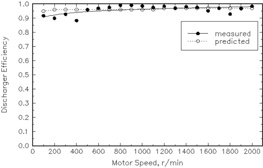
Figure 4.19(ii) Boost discharger efficiency in discharging mode.
