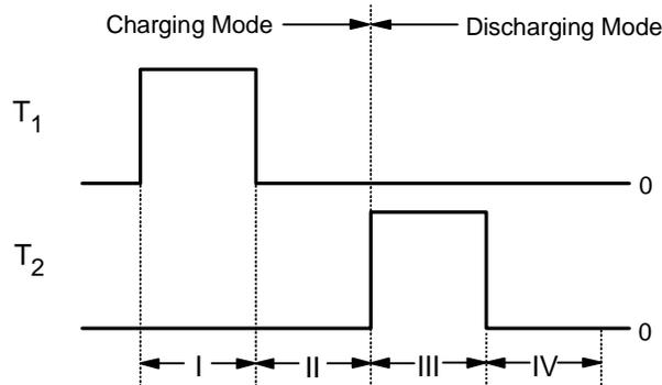
Figure 4.10 Four operational modes of the proposed charger/discharger.
