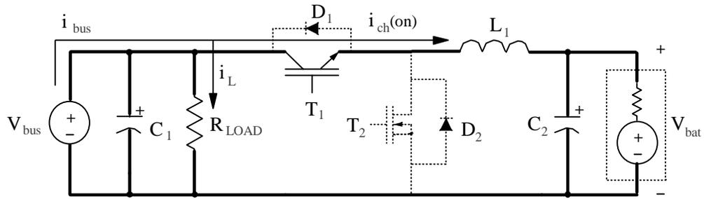
Mode I:  $T_1$  on and  $T_2$  off (charging mode)
