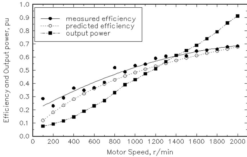
Figure 4.17(ii) Overall system efficiency and normalized output power in charging mode without PFC preregulator.
