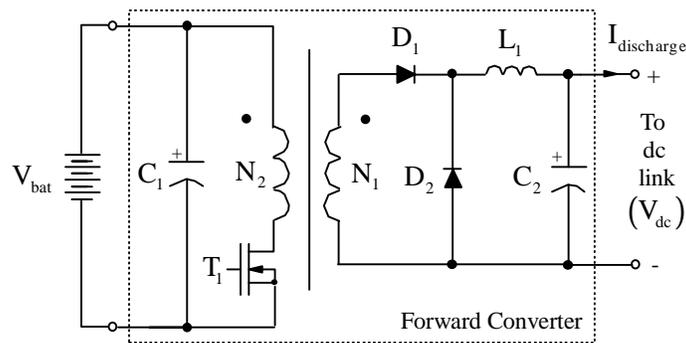
Figure 4.7 Forward converter as a discharger.
