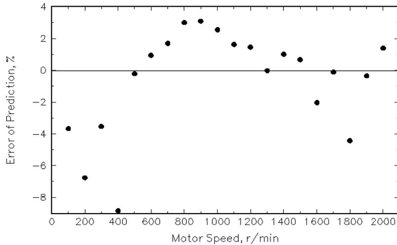
Figure 4.19(iii) Efficiency prediction error versus SRM speed for boost discharger in UMD system.
