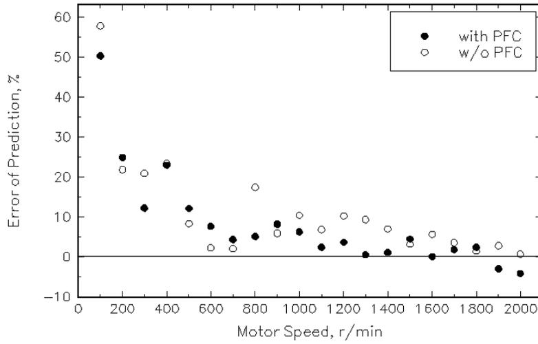
Figure 4.18 Error of prediction of the SRM-based UMD system efficiency with and without the PFC at charging mode.
