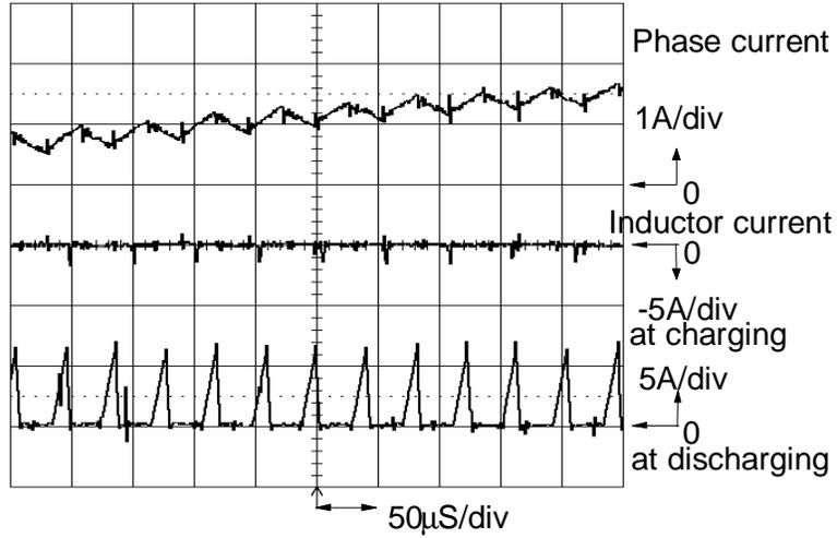
Figure 4.15 Current waveforms of SRM phase and inductor in charger/discharger at 1,000r/min.
