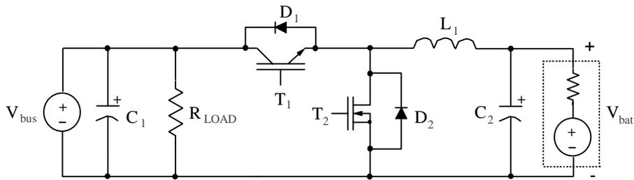
Figure 4.9 Simplified circuit diagram of the proposed charger/discharger.
