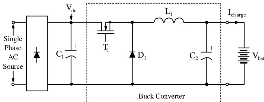
Figure 4.3 Diode bridge rectifier with a buck converter.
