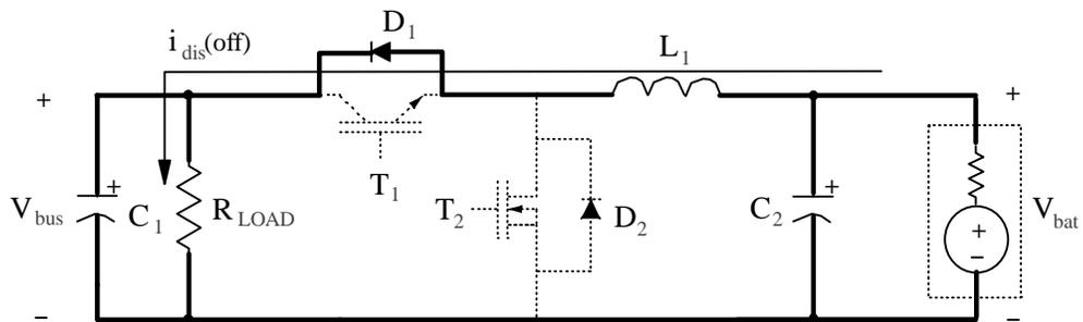
Mode IV:  $T_2$  and  $T_1$  off (discharging mode)
