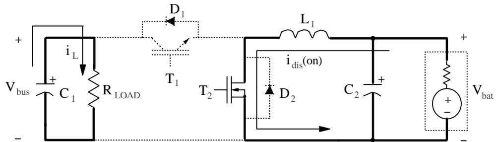
Mode III:  $T_2$  on and  $T_1$  off (discharging mode)
