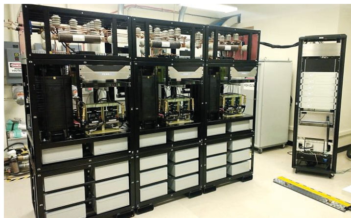
Figure 1-6: Medium-voltage impedance measurement unit developed by CPES in 2014
