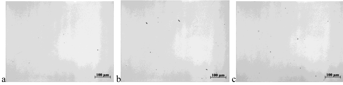
Figure 2.10: Raw optical images of a) group 1, b) group 2 and c) group 3 samples showing some of the observed defects.
