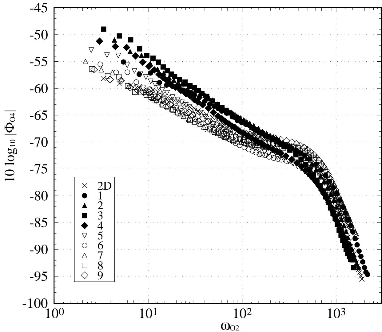
**Figure 63.** Spectral power density of  $p$  ( $Re_\theta = 23400$  (2-D); 23200 (3-D)) normalized using  $Q_e$  as the pressure scale and  $\delta^*/u_\tau$  as the time scale. The numbers in the legend denote the measurement station.
