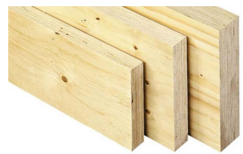
Fig. 52 LVL panel photo (Green & Karsh pg. 39).
