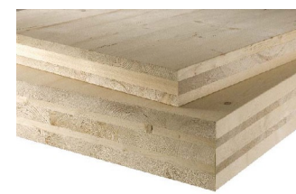
Fig. 2 CLT Photo (Green & Karsh pg. 37)
