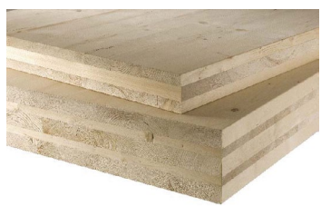
Fig. 51 CLT panel photo (Green & Karsh pg. 37).
