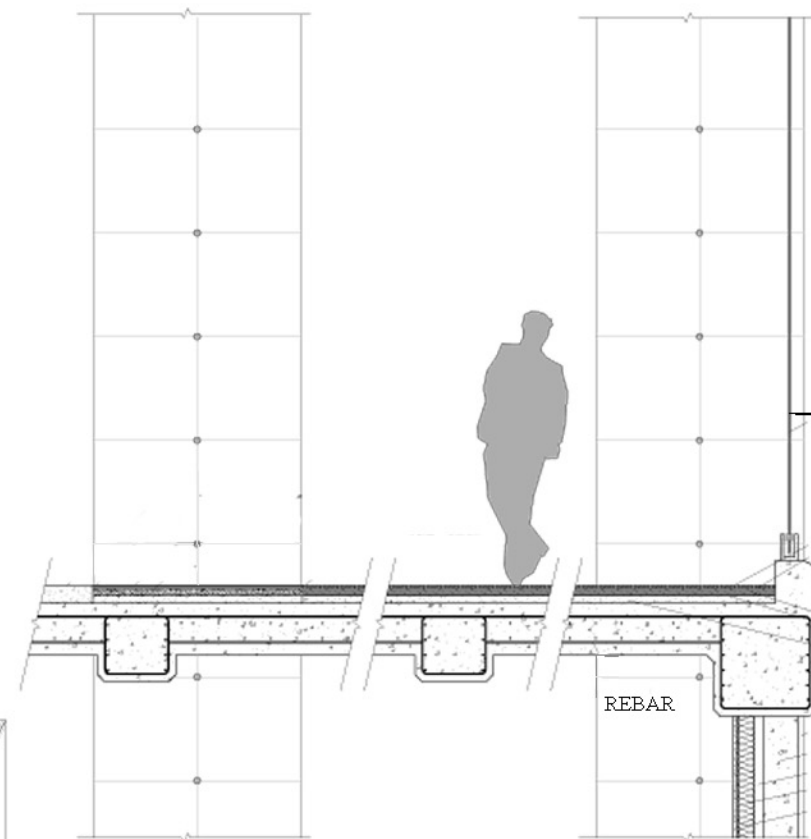
INTERIOR EXHIBIT HALL FLOORING AND STRUCTURE DETAIL
