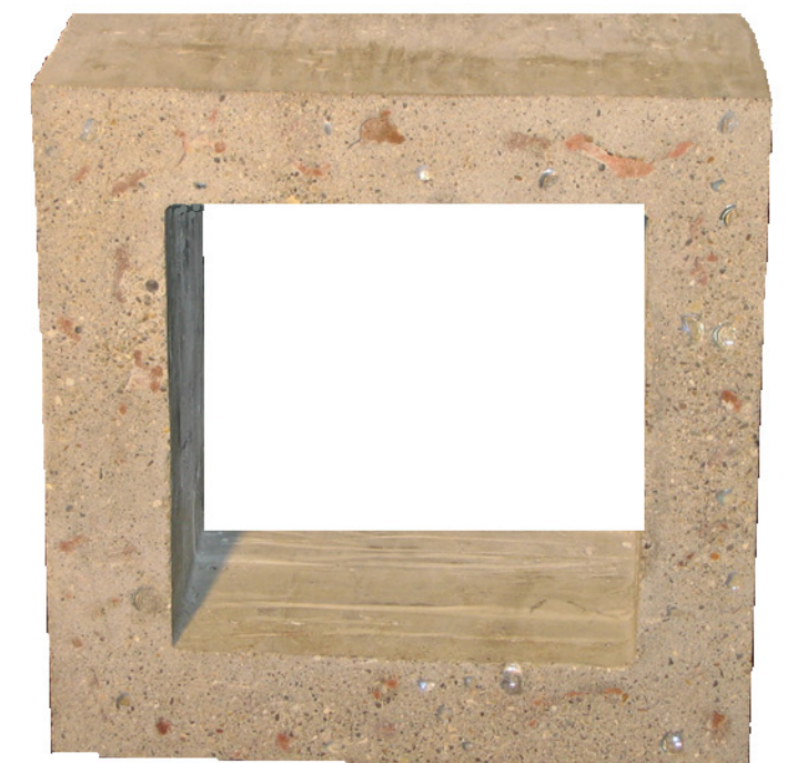
PHOTOGRAPHS OF SOUTH AND WEST CUSTOM WALL BLOCK MOCK-UP SHOWING THE IN-BEDDED GLASS AND RED LAVA ROCK
