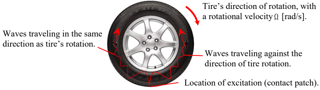
Figure 2.14. Wave interaction with the rotation of the tire.
