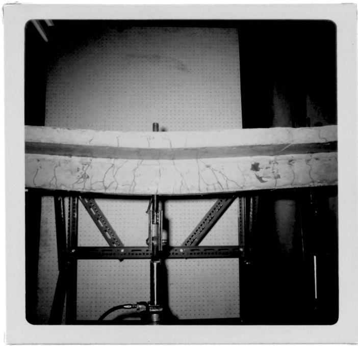
Figure 11. Center Crack Pattern
