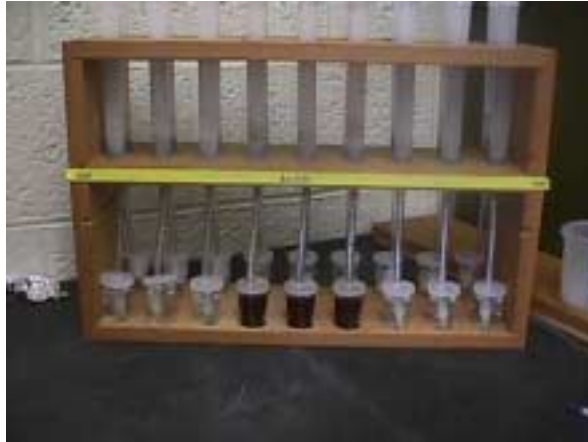
Figure 2.2 Example of one of the racks of 18 columns, with vials to collect the leachate.
