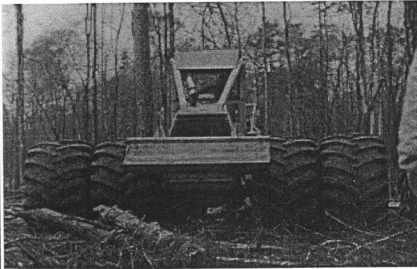
Figure 1.1. A skidder equipped with experimental ultra-wide tires (dual 43-inch wide-tires).
