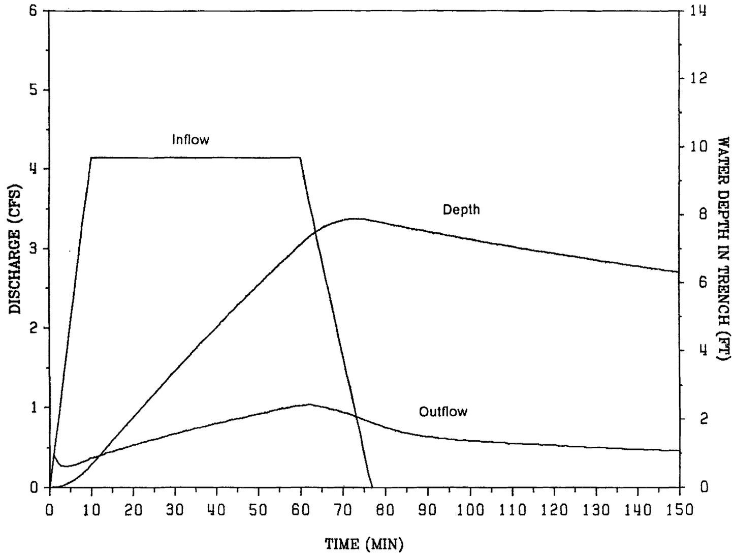
Figure 1 . Results of hydrologic routing in an infiltration trench
