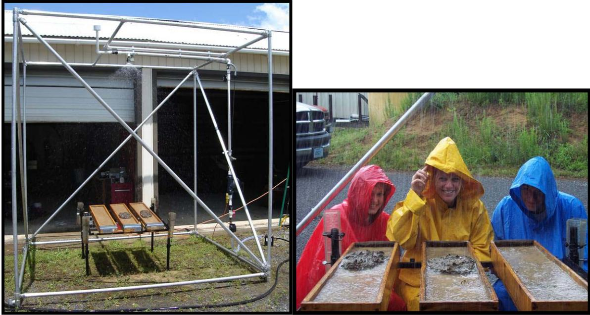
**Figure 5.2. Tlaloc 3000 portable rainfall simulator was used to apply rain to the box plots and samples were collected from the base of the plots 10, 20, and 30 minutes after the onset of runoff.**
