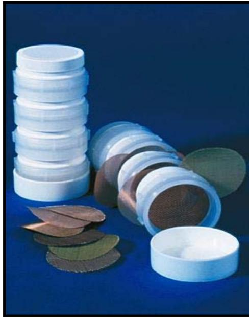
**Figure 3.1. Mini-Sieve Microsieve Set used to separate particles in runoff into 63 and 500  $\mu\text{m}$  particle size categories.**
