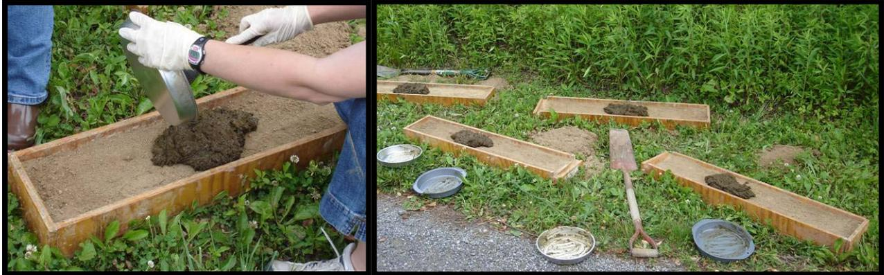
**Figure 5.1. Application of a standard cowpat to portable box plots packed with three different Virginia soils.**
