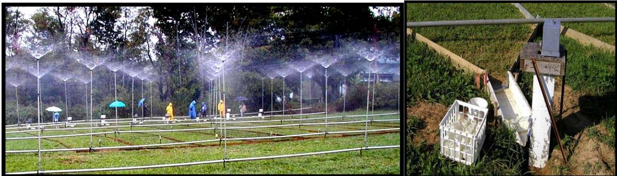
**Figure 6.1. Portable rainfall simulator was used to apply rain to the transport plots and samples were collected from the base of the plots every 10 minutes after the onset of runoff.**
