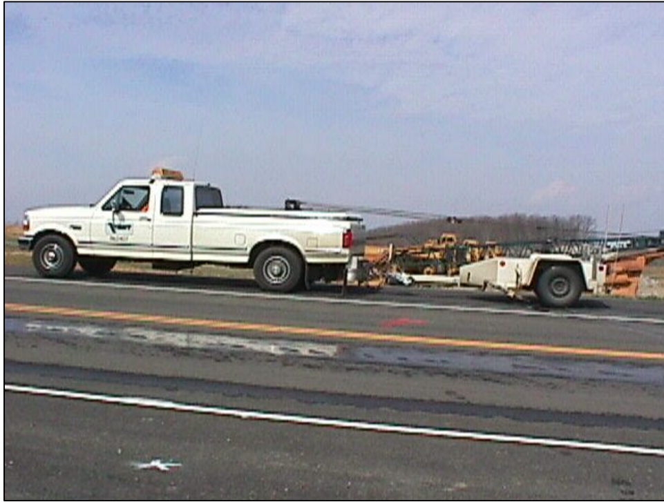
Figure 2.2 VDOT Locked Wheel Skid Trailer
