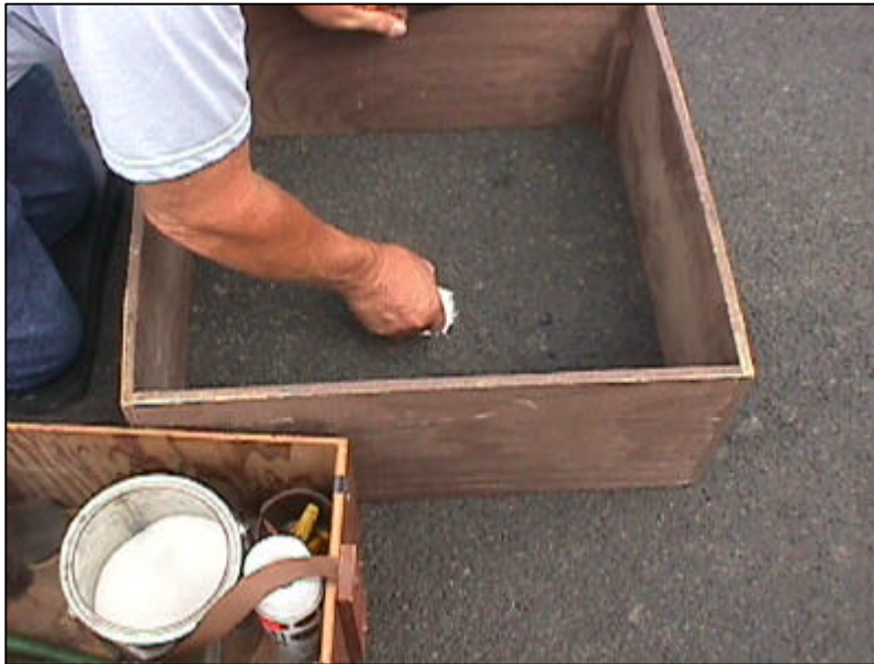
Figure 2.5 Sand Patch Test
