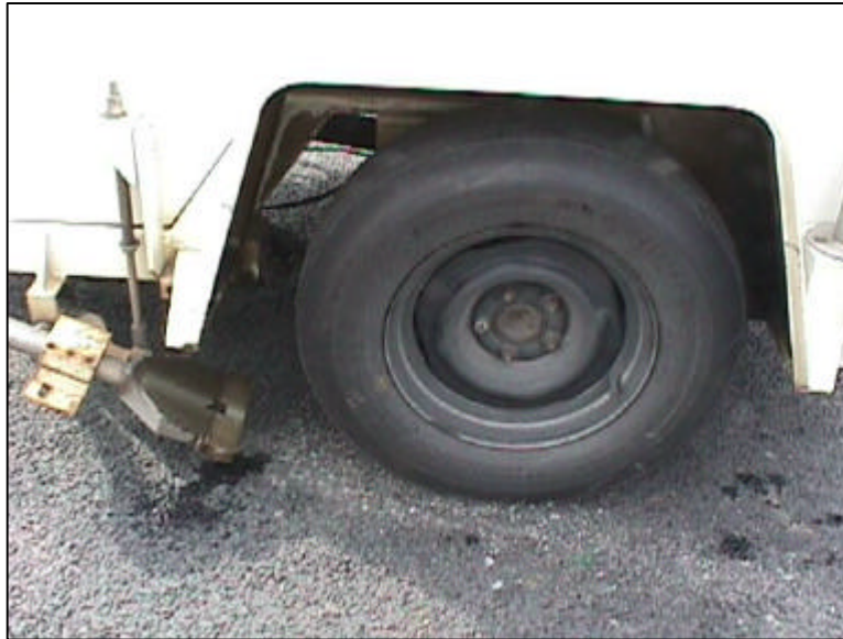
Figure 2.3 Water Dispensing System and Tire of Locked Wheel Skid Trailer
