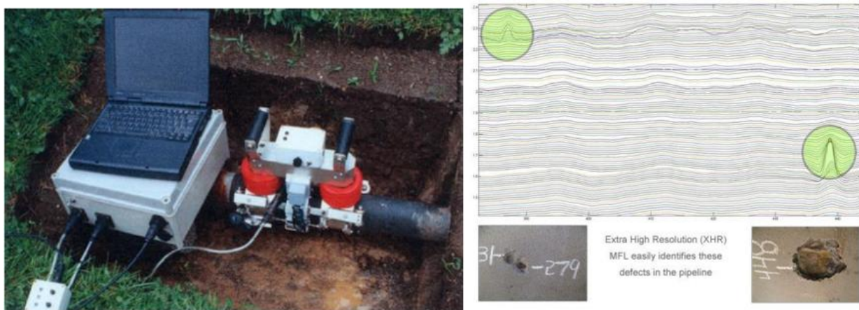
Figure 2-11: Left shows a Full Circumferential Pipe Wall Inspection Tool. Right shows Contour Map Showing the Flux Density from Hole Defect. (Courtesy of PURE Technologies)
