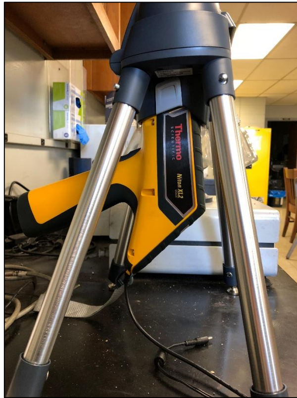
Figure 11. Thermo Scientific Niton XL2 GOLDD in analysis cradle
