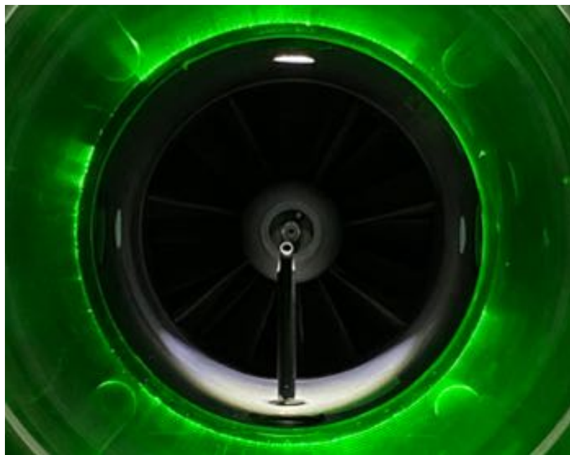
Figure 3.6: Particle Sampling Probe Upstream of the Engine Inlet
