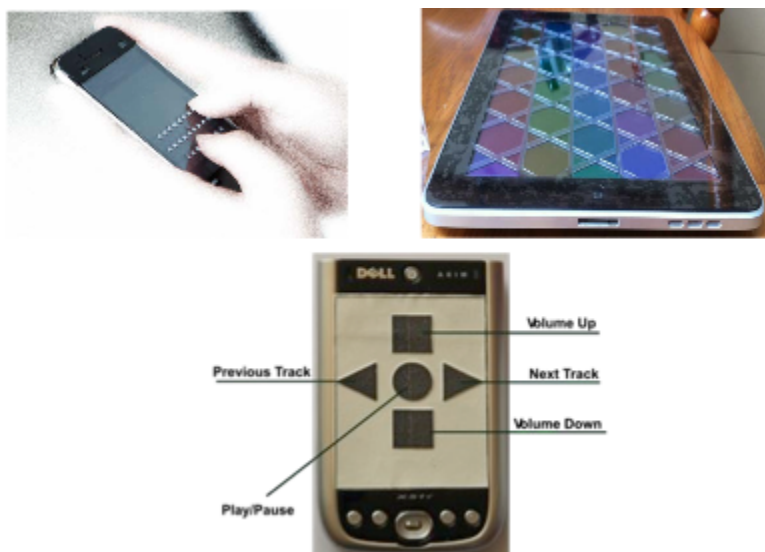
Figure 2.2: Left: Tactile keyboard [8]. Right: Tactile grid [3]. Bottom: Overlay for MP3 player [63].
