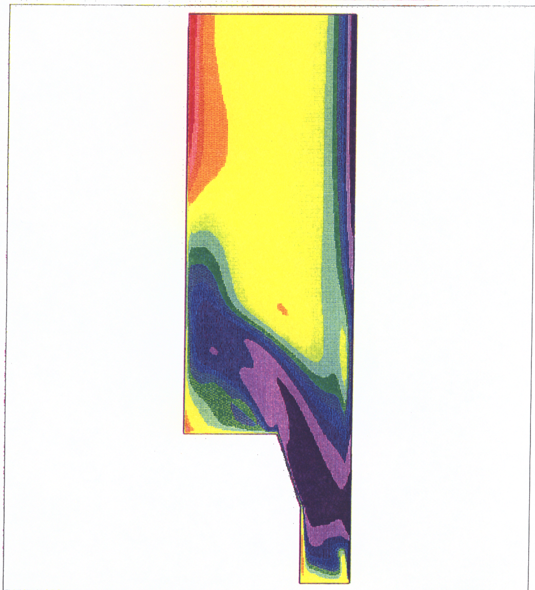
Figure 19. Quarled Burner Case 2, Percent Change Eddy Viscosity from the Standard k-epsilon Model to the Chen Modification
