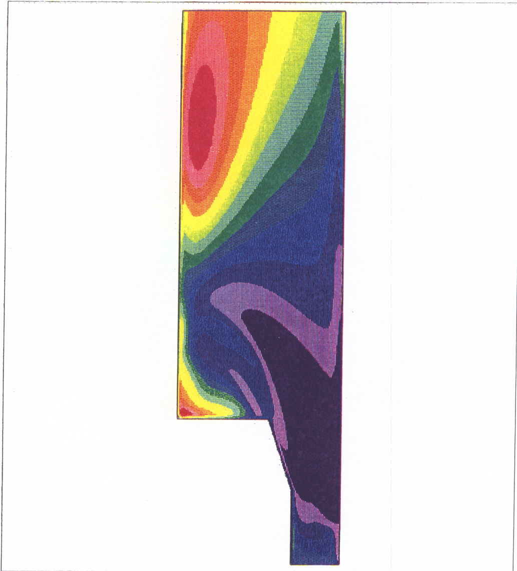
Figure 26. Quaried Burner Case 2, Percent Change Turbulent Kinetic Energy from Standard k-epsilon to Chen Modification
