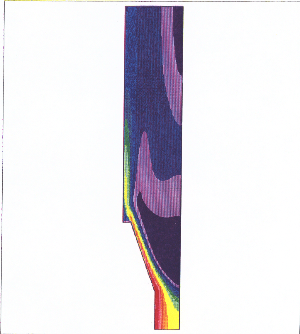
Figure 13. Quarried Burner Case 1, Velocity Magnitude Predictions with the Chen Modification
