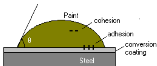
Figure 1.3 Schematic of a paint drop applied onto a coated-steel surface. \theta is the contact angle at equilibrium state.
