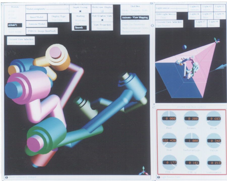
Figure 33. 7-R Mechanism with Visible Collision
