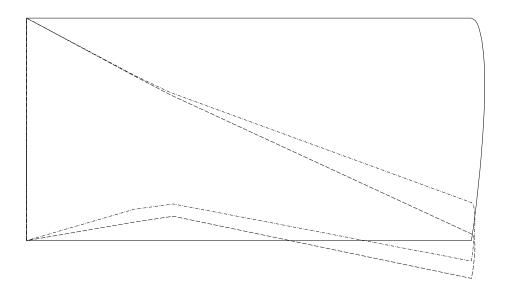
Figure 6.14: Initial and final optimized wing planforms.
