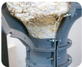
Mold failures during compression.
