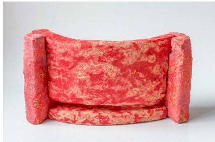
Shellac paint prototype after initial coat of pigmented shellac (left) and first round of sanding (right).
