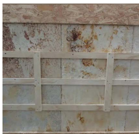
Mycelium drywall insulation, Grown Bio by Ecovative
