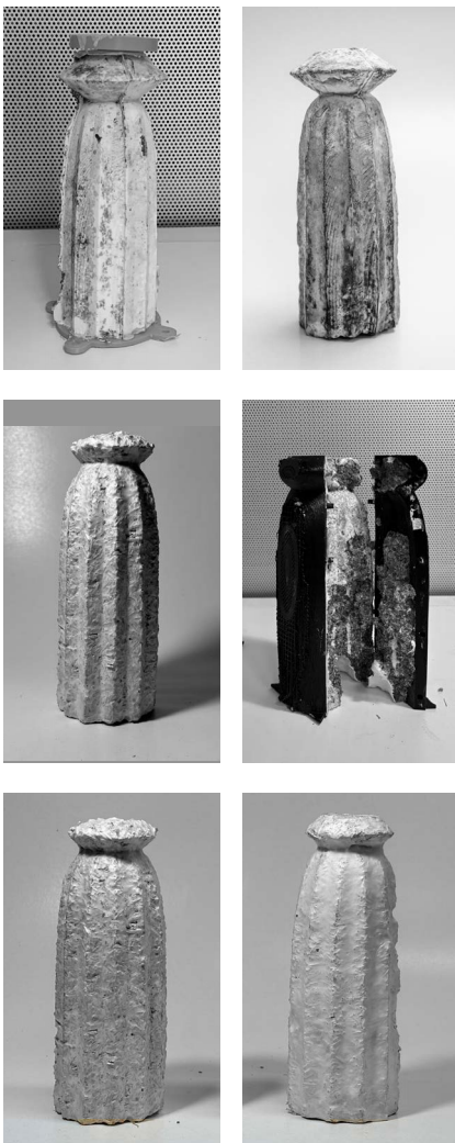
Rapid prototyping of luminary design V1 revealed many conflicting features of the design and material.
