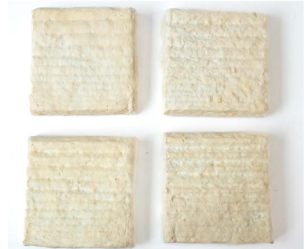
Oyster mycelium samples containing 30% (left) and 20% (right) hemp.
