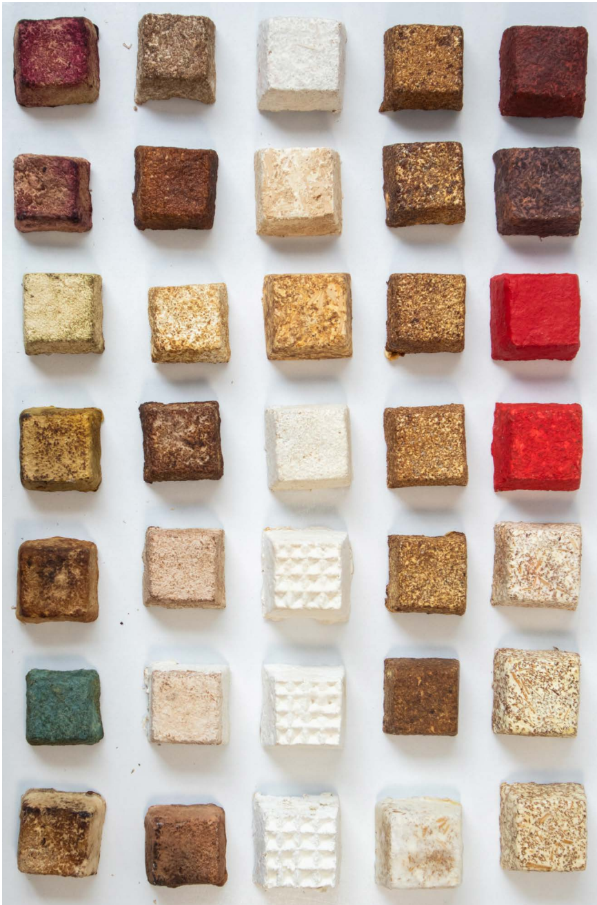
MBC swatches treated with various dyes and coatings.
