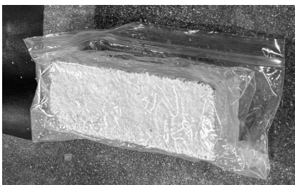
Samples drying in dehydrator (top) and sample rehydrating with controlled moisture content (bottom)
