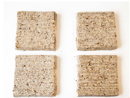
Samples that experienced contamination during growth.
