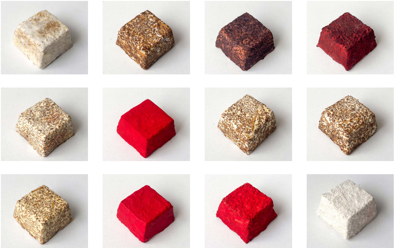
MBC swatches treated with various coatings and dyes.
