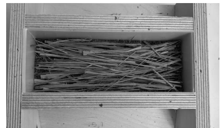
Coconut coir, soybean roving, and bamboo fiber layers during molding.
