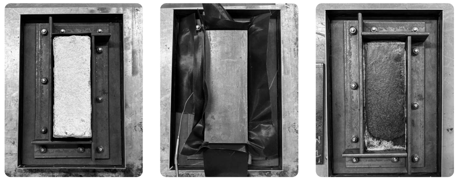
Sample during pressing, from left to right: uncompressed, post cold pressing, post hot pressing.
