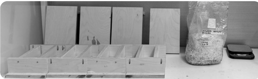
Plywood molds and mycelium spawn on laminar flow hood bench.
