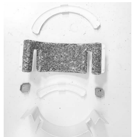
Upper luminary component during demolding.
