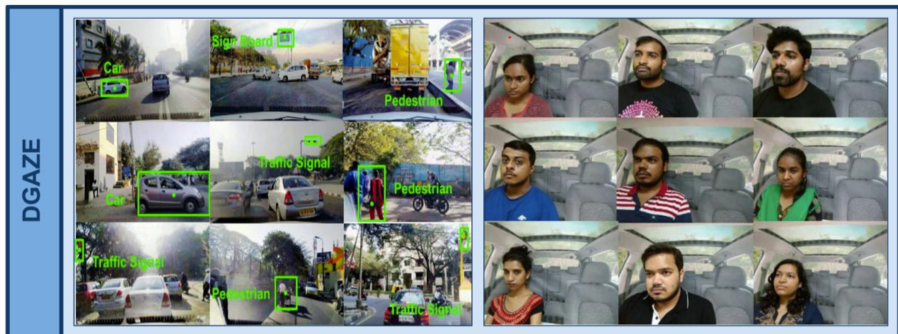
Figure 3.1: Showcases DGAZE, a dataset designed to capture driver gaze on the road by incorporating both driver and road view through the use of inexpensive mobile phone cameras (Figure credit: [4]).
