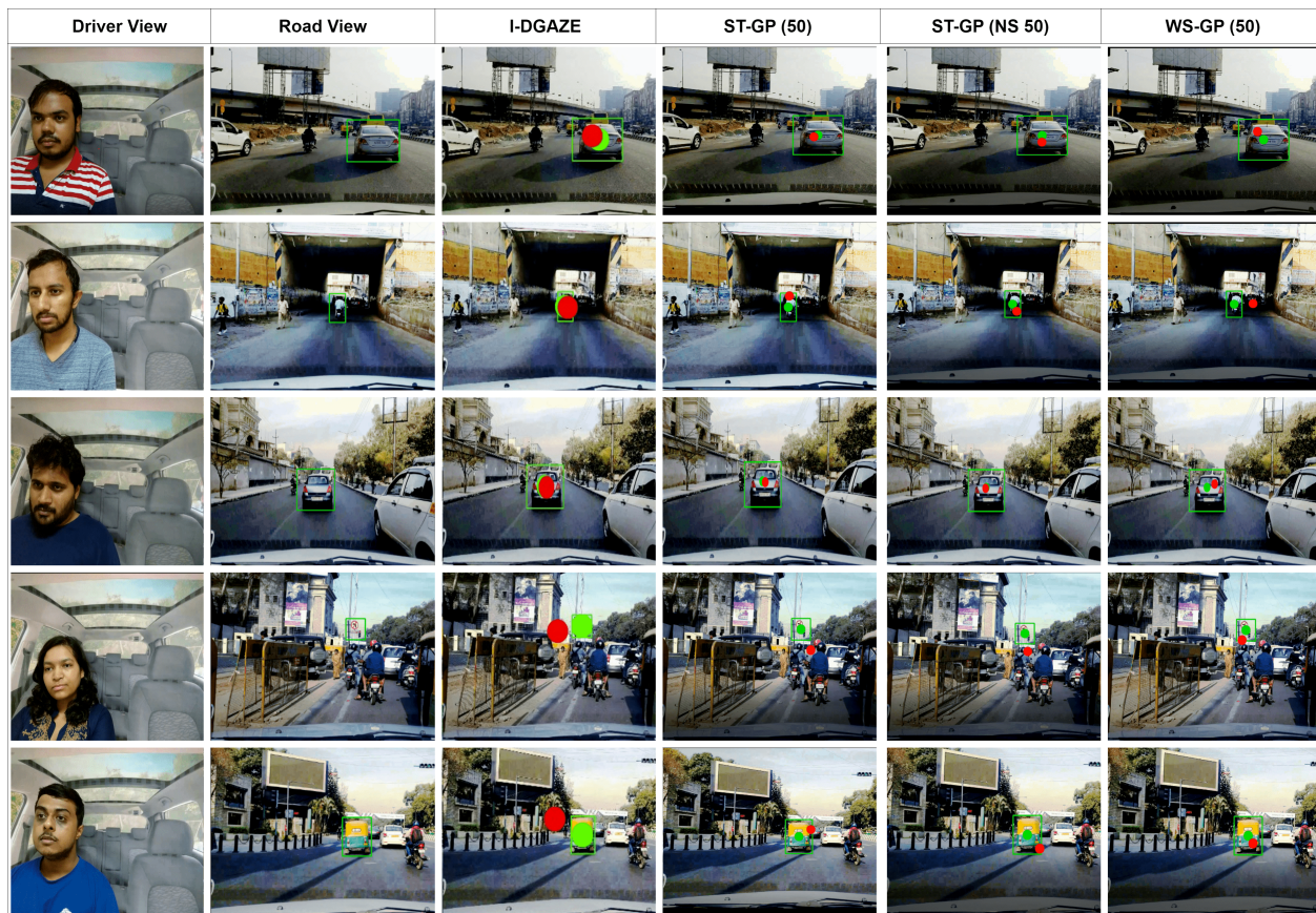
Figure 5.3: Qualitative analysis of estimated gaze points using three top-performing models (ST-GP (50), ST-GP (NS 50), and WS-GP (50)). The figure is organized into columns displaying driver images, road images, and ground truth gaze points (green circles) alongside estimated gaze points (red circles) for each model. The proximity of red and green circles indicates the performance of each model.
