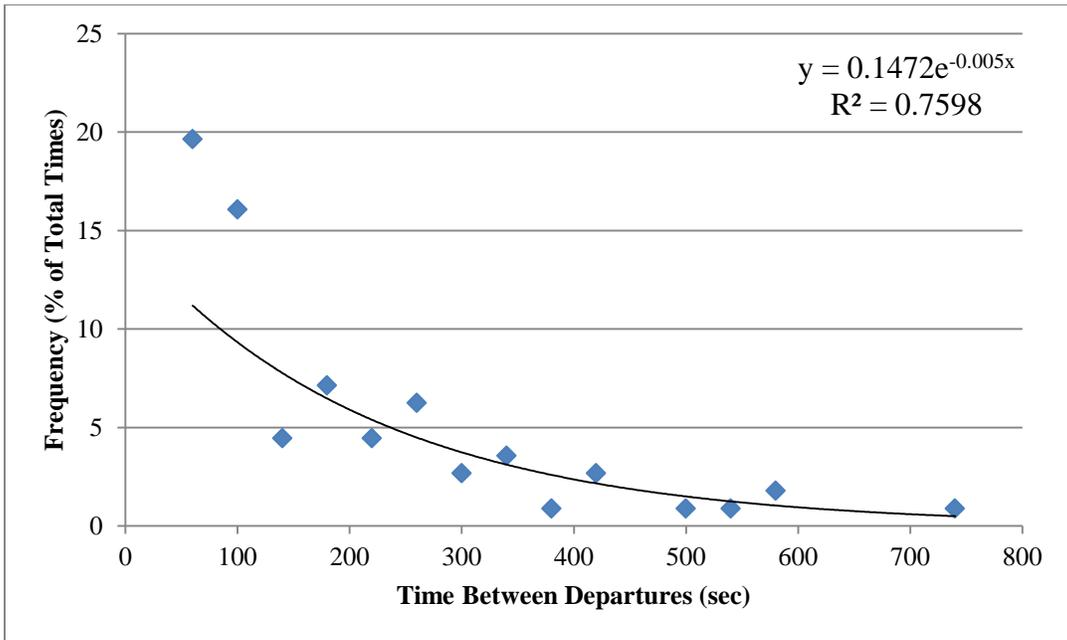
Figure A-6: Overall Service Distribution with 2 Loaders in Operation
