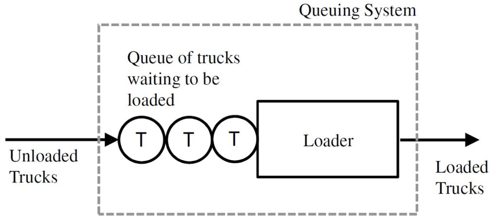
**Figure 3.3: Truck and Loader Queuing System**
