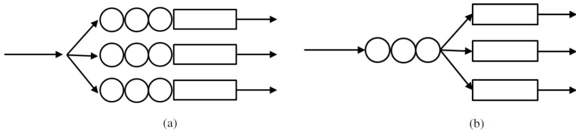
Figure 3.2 Multichannel Queuing Systems
