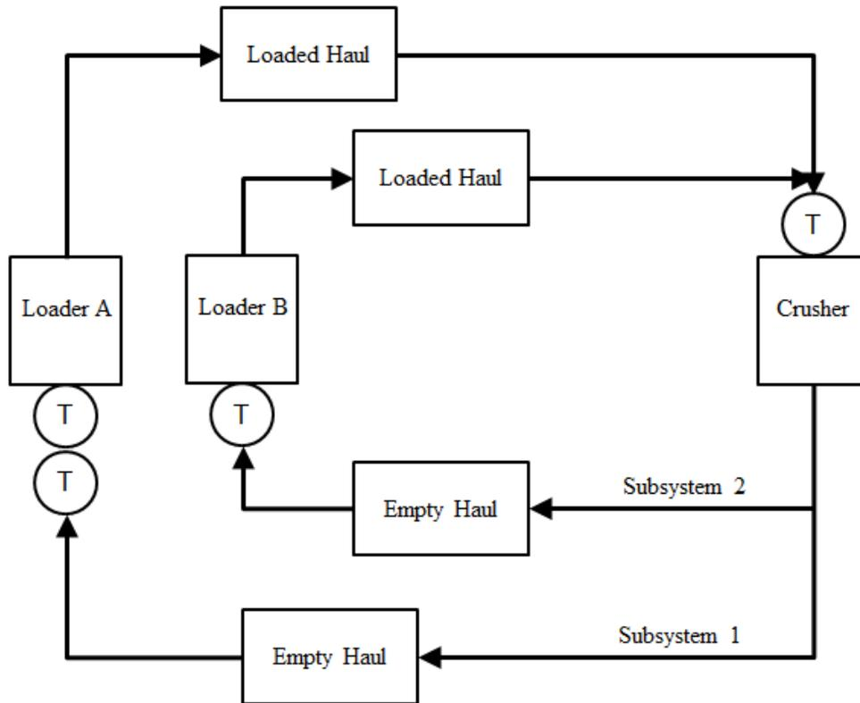
Figure 3.7: Queuing Schematic with Multiple Pits
