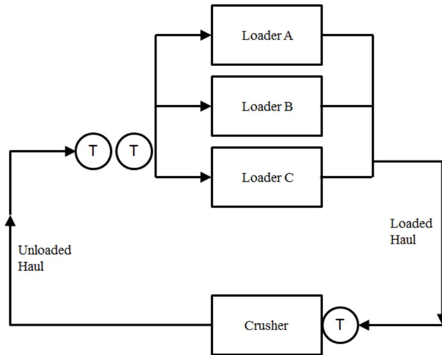
**Figure 3.5: Cyclic Queuing System with Parallel Loaders**
