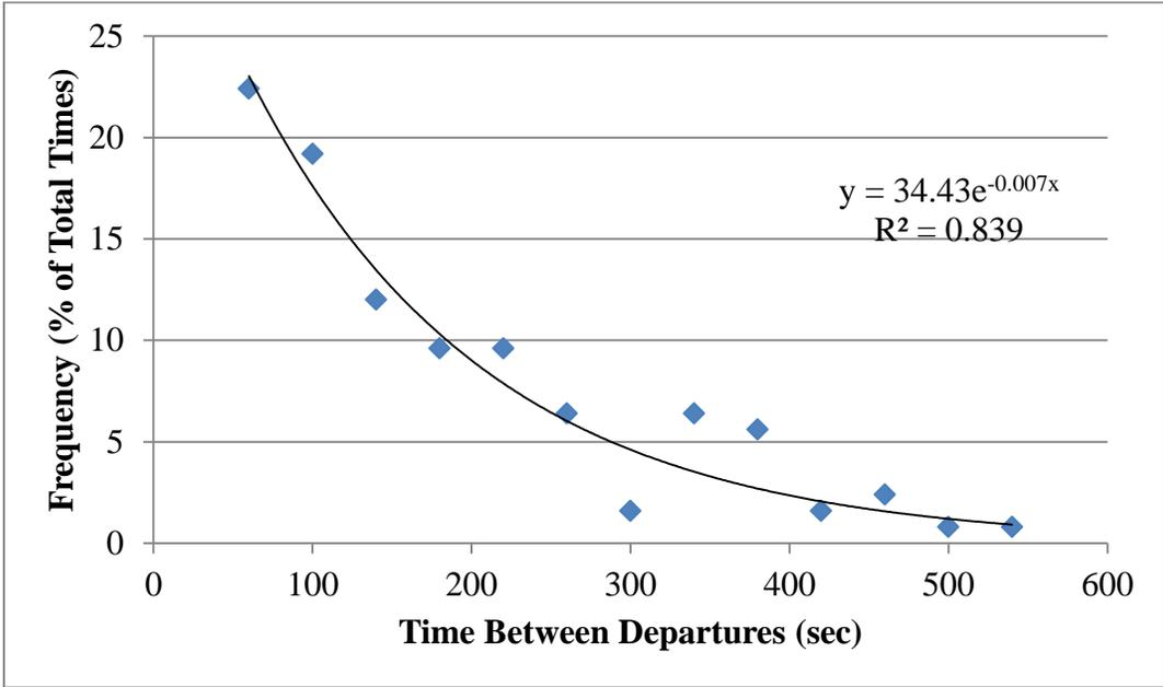
Figure A-5: Overall Service Distribution with 3 Loaders in Operation
