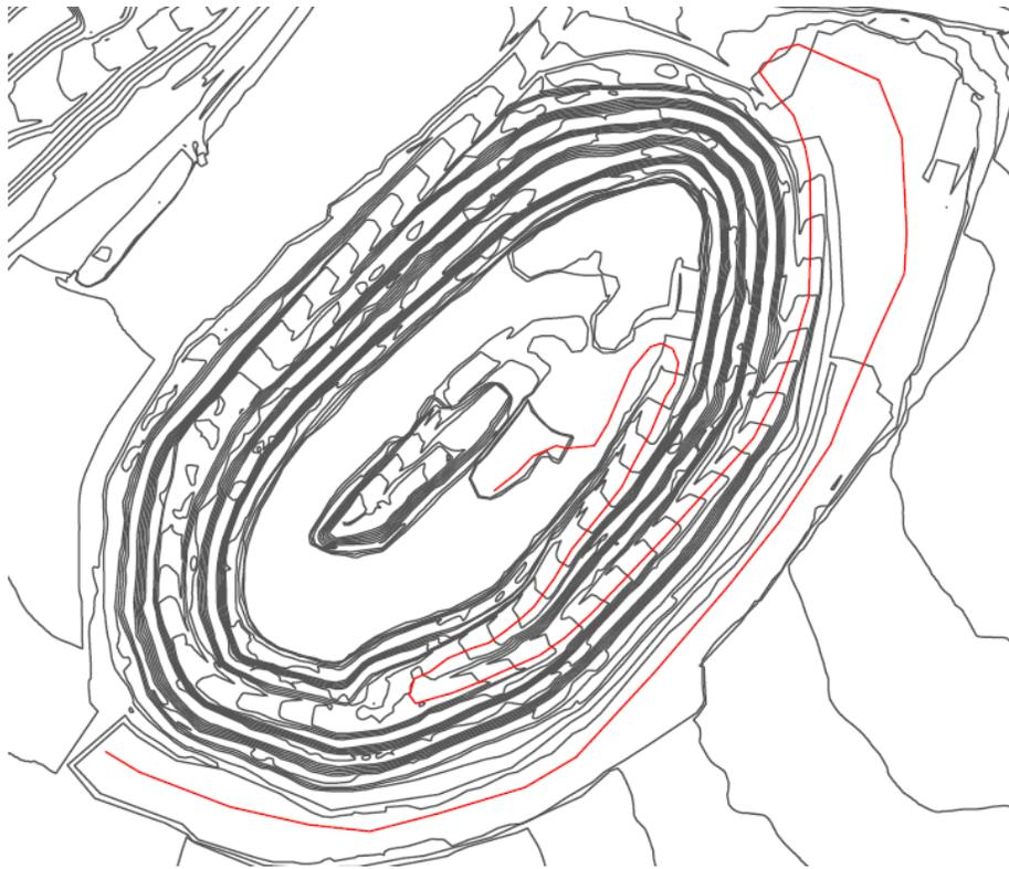
**Figure 3.13: Haul Route from Pit to Crusher**
