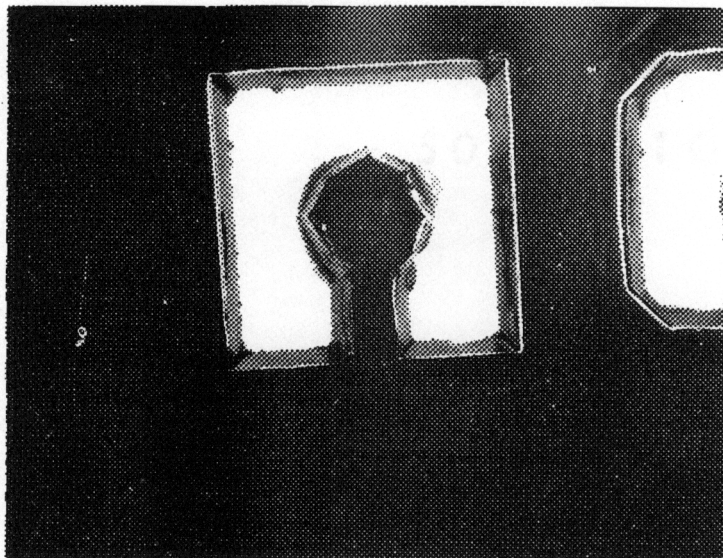
Photograph 3-5. Part "B": Total corner erosion (8x magnification).
