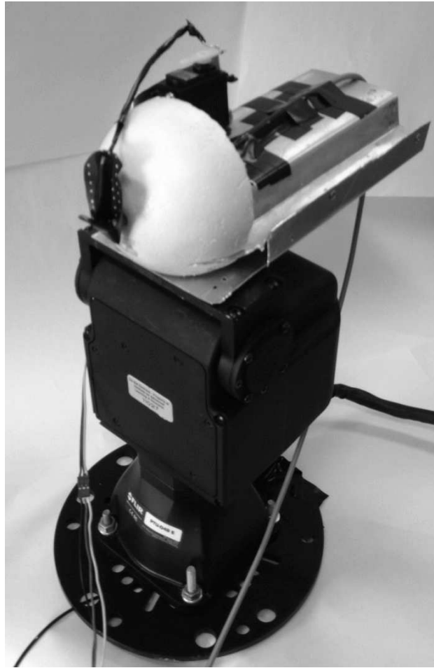
Figure 3.3: Actuation setup mounted on the Pantilt unit.
