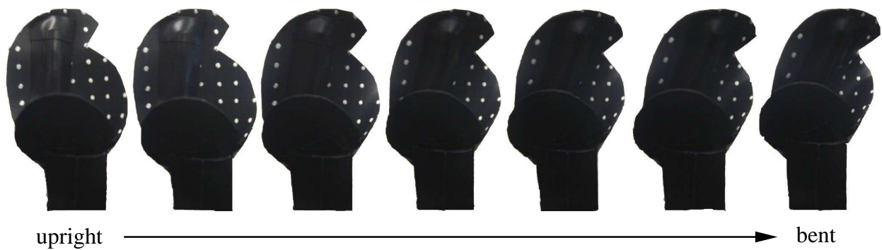
Figure 3.2: Seven shape changes from upright to bent configuration in the ear prototype.
