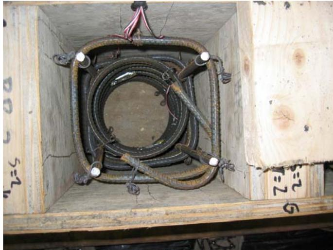
Fig. 3.2 Specimen Reinforced with Spiral and Ties
