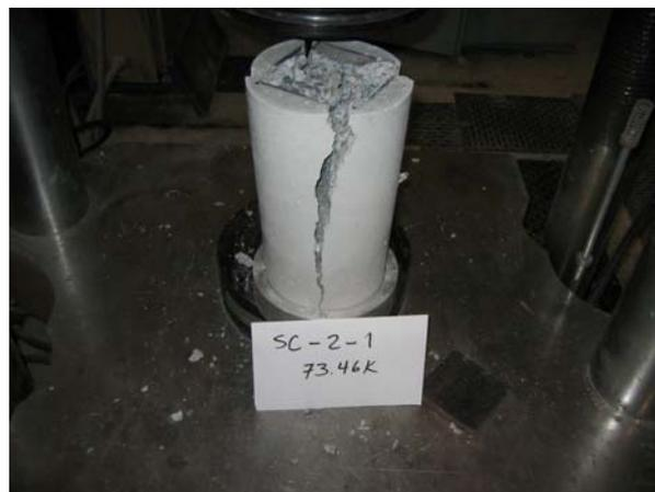
Fig. 5.5 Cylinder Block at Failure  $A/A_b=2$
