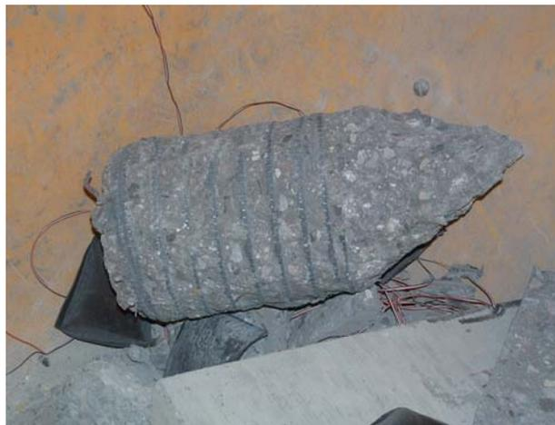
Fig. 5.27 Failure Cone in Specimen Failed in the Base.
