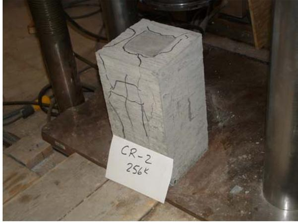
Fig. 5.25 Typical Failure in the General Zone Showing Plate Indentation.
