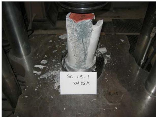
Fig. 5.7 Failure of Cylinder Block with  $A/A_b=1.5$  (Hexagonal Plate).
