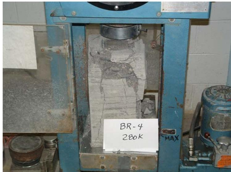
Fig. 5.24 Typical Failure in the General Zone.
