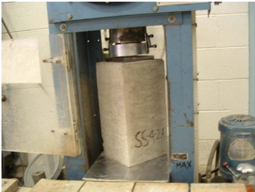
Fig. 3.1 Test Setup for a Square Prism
