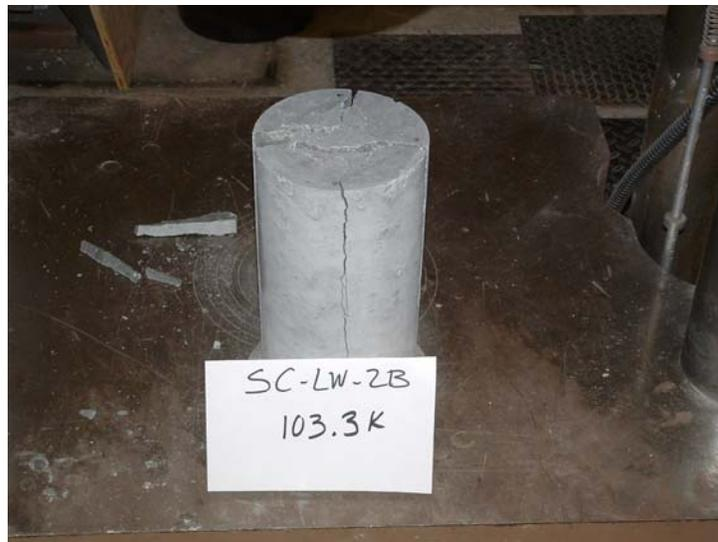
Fig. 5.14 Failure of Cylinder Block with  $A/A_b = 2$  (Square Plate).
