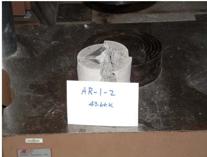
Fig. 5.11 Failure of cylinder block with aspect ratio = 1.
