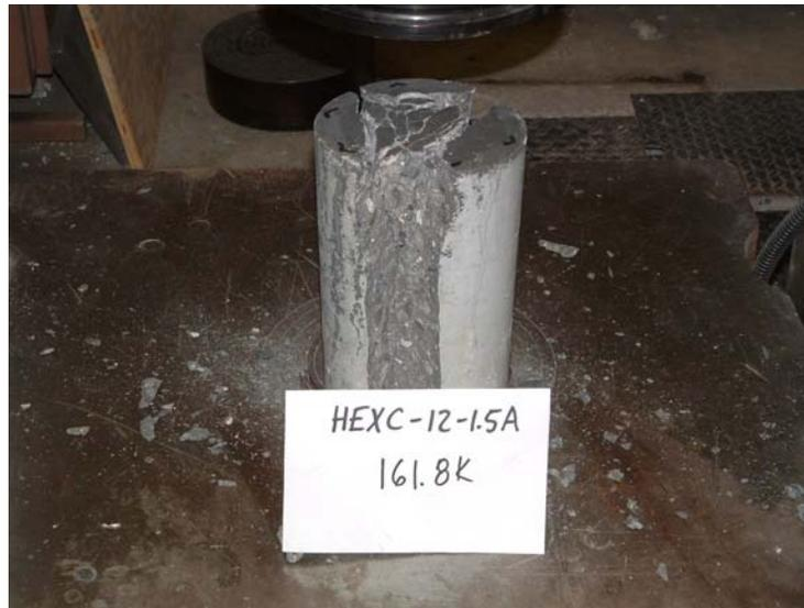
Fig. 5.17 Failure of Cylinder Block with  $A/A_b = 1.5$  (Hex Plate).
