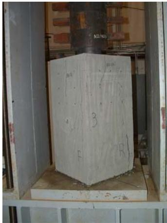
a) Test Setup with Specimen at Failure
