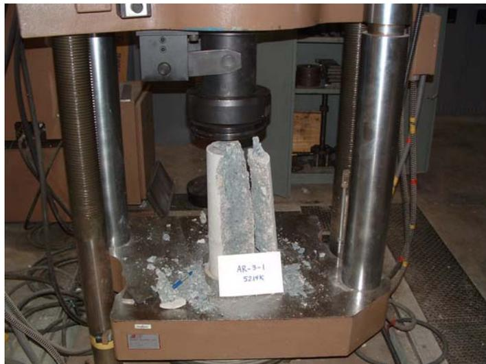
Fig. 5.10 Failure of Cylinder Block with Aspect Ratio = 3.
