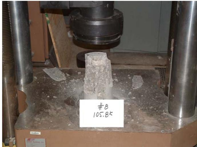
Fig. 5.19 Failure of Cylinder Block with Duct Size of 2.375 in.
