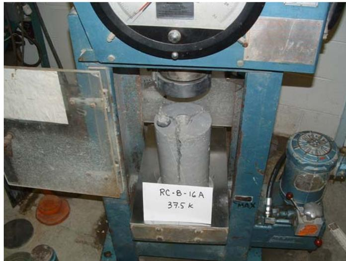
Fig. 5.16 Failure of Cylinder Block with  $A/A_b=16$  (Round Plate).
