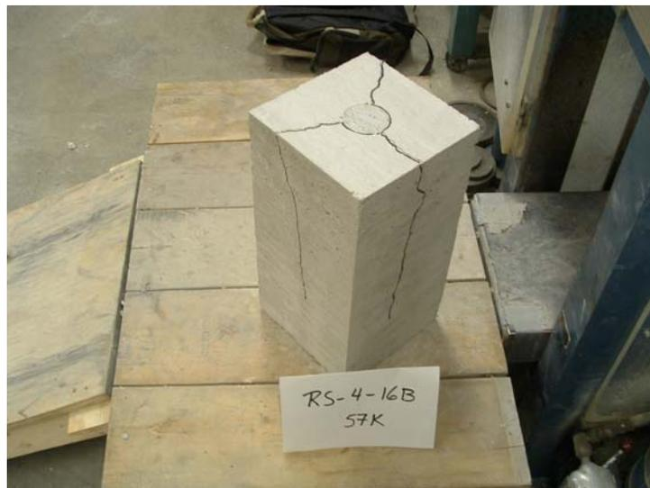
Fig. 5.1 Failure of Square Block Loaded with Round Plate,  $A/A_b=16$ .
