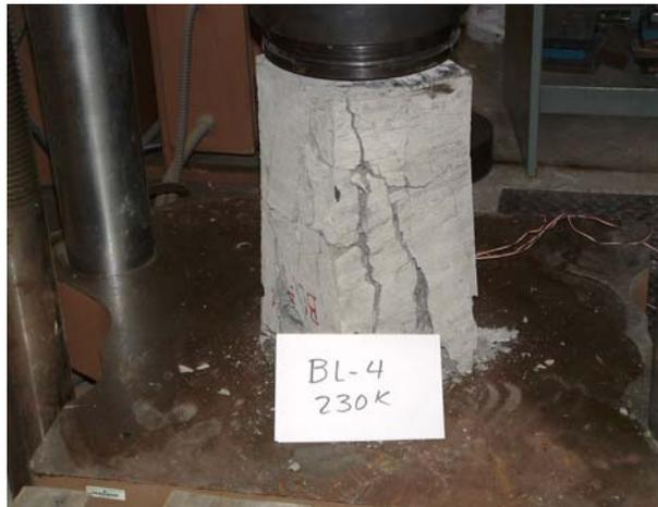
Fig. 5.26 Failure in the Base of the Prism
