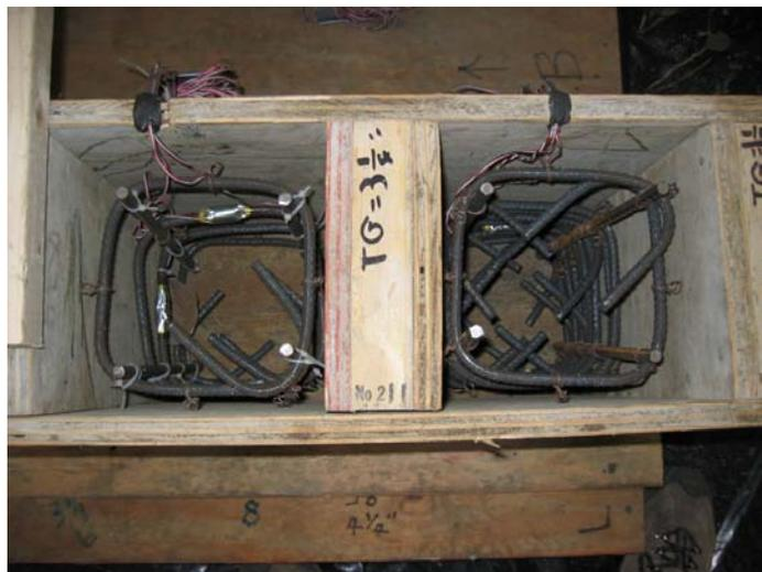
Fig. 3.3 Specimens Reinforced with Ties
