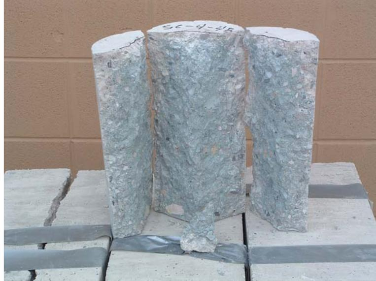
Fig. 5.2 Failure of Cylinder Prism Loaded with Square Plate,  $A/A_b=4$ .
