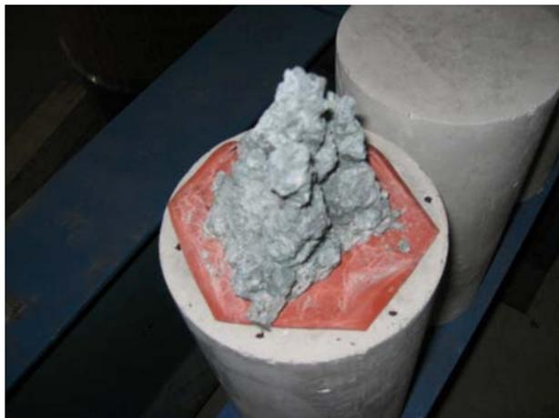
Fig.5.8 Typical Failure Pyramid from Cylinder in Fig. 5.7.
