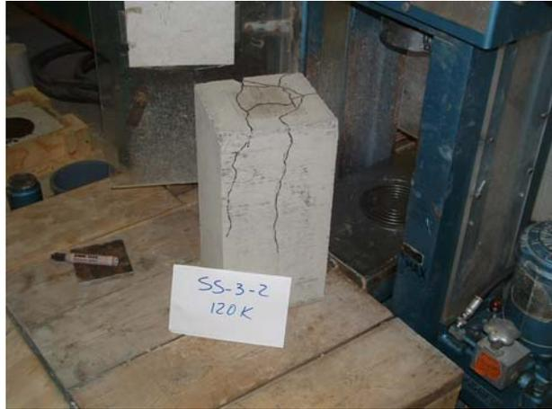
Fig. 5.6 Square Block at Failure  $A/A_b=3$
