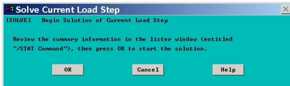
**Note:** The loads specify in this analysis is higher than the expected ultimate load of the beam. Therefore, the program will not terminate when the solution is done. The user has to stop the nonlinear analysis when the solution has converged, the ultimate load has been reached, and the load being applied is decreasing.
