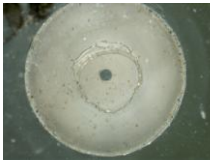
Figure 3-21 Sol-gel bonded diaphragm and ferrule
