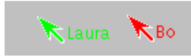
Figure 2.3: A telepointer indicates a remote participant’s cursor location in the workspace. Typically, each user has a unique color. Shapes and names may also be used to distinguish users.
