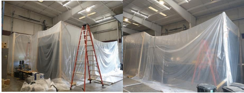
Figure 3.11. Enclosure around the test rig
