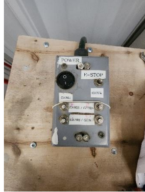
Figure 3.2. Controller for operating the test rig.
