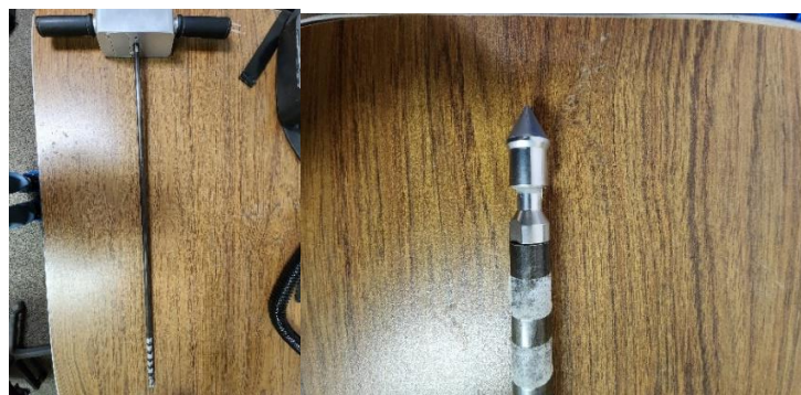
Figure 3.9. Humboldt HS-4210 Digital Static Cone Penetrometer
