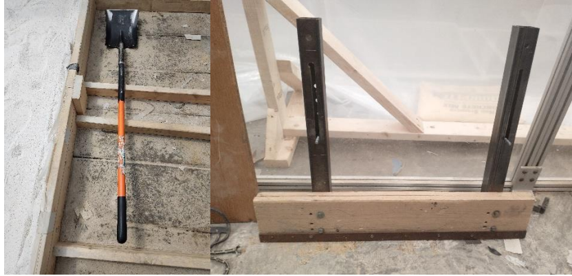
Figure 3.8. Shovel and leveller used for soil preparation.
