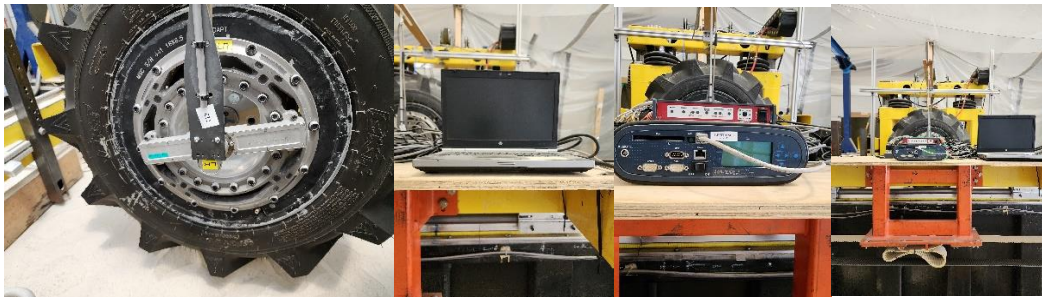
Figure 3.3. MSC LW 12.8-45 sensor with data acquisition system
