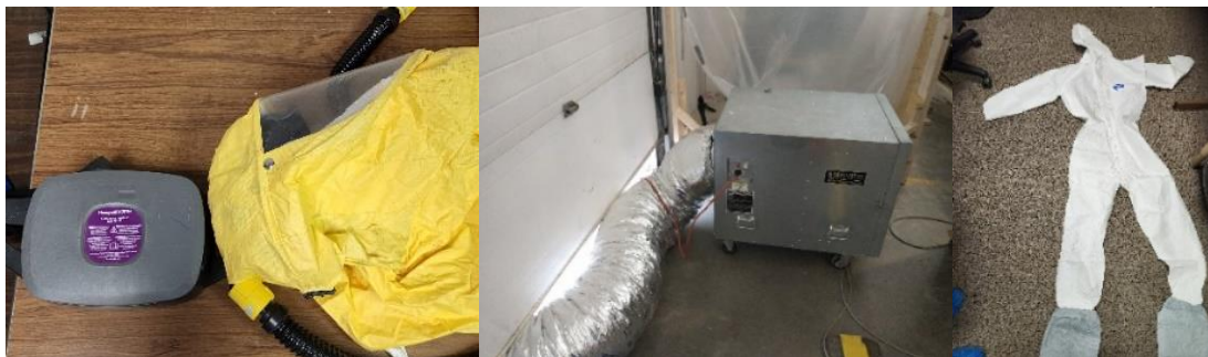
Figure 3.12. Safety Equipment used. (a) PAPR (b) Negative air machine (c) Tyvek suits
