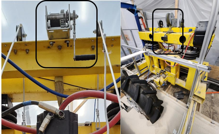
Figure 4.5. Wheel lowering mechanism.
