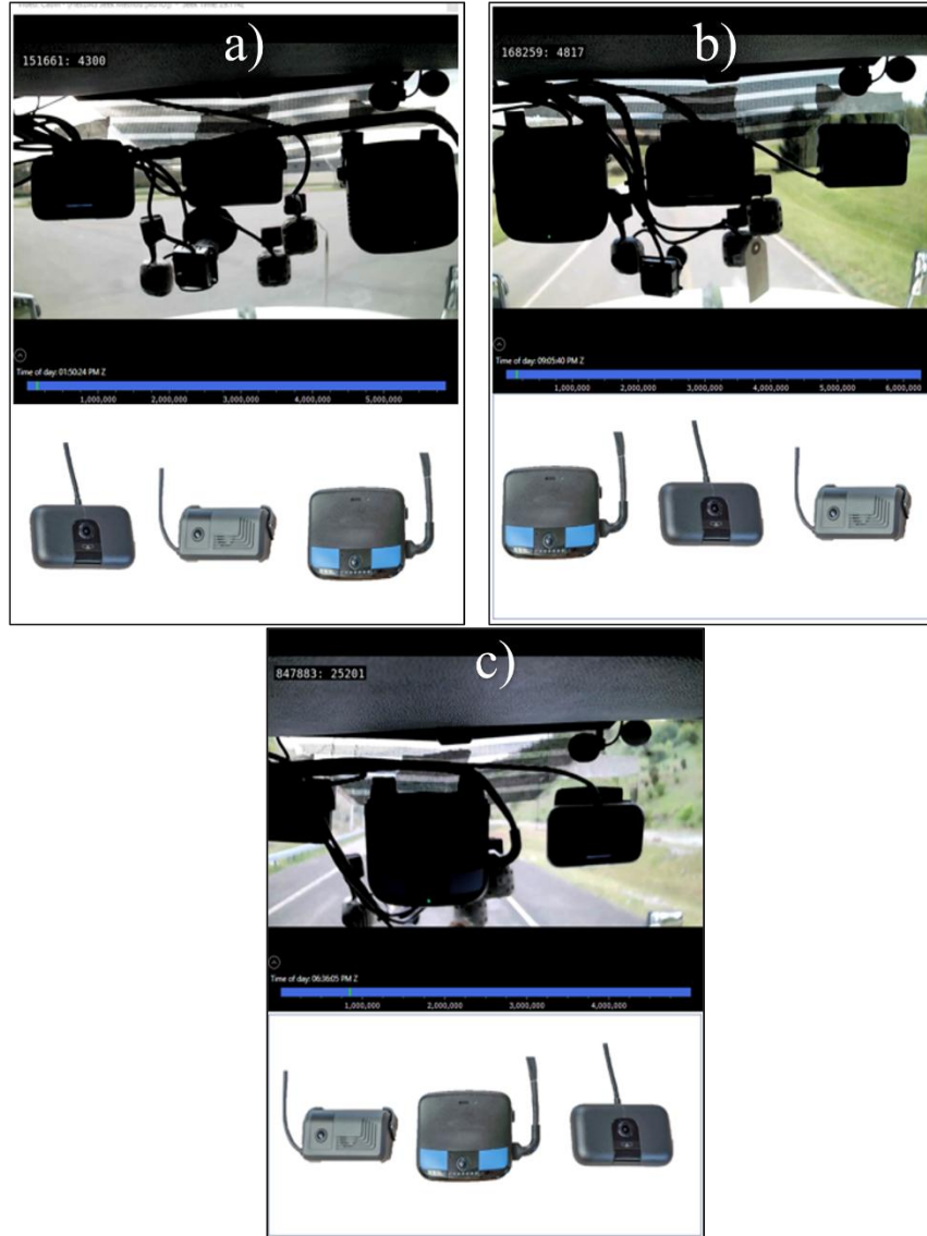
Figure 4 - The three rotations used during testing: (a) Rotation 1: Motive, Samsara, Lytx; (b) Rotation 2: Lytx, Motive Samsara; (c) Rotation 3: Samsara, Lytx, Motive.
