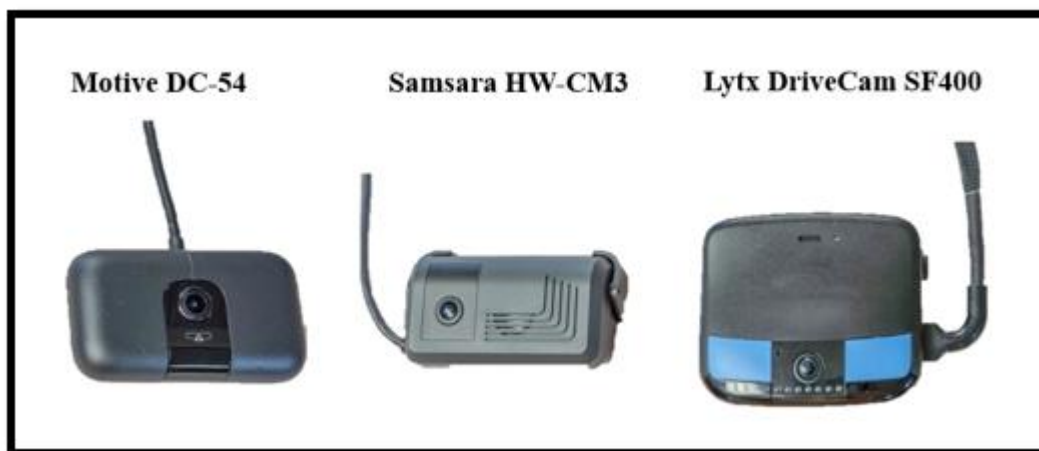
Figure 1 - The three DMSs used for benchmarking (Left to right: Motive, Samsara, and Lytx.)
