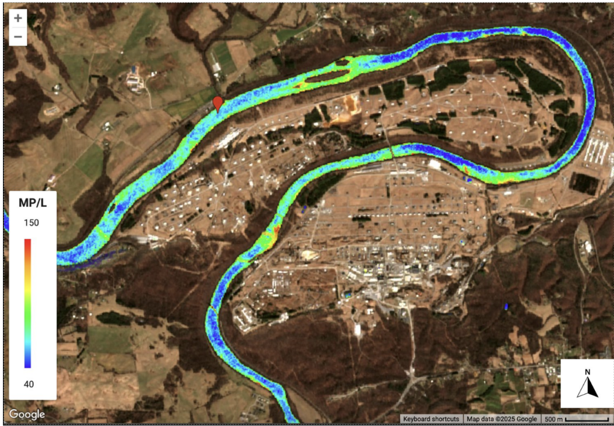
Figure 13: Example Sentinel-2 image showing average MP concentration proxy values along the New River, VA during the winter of 2023-2024. The color bar is linearly stretched from 40 to 150 MP/L. The Red pin denotes where the time series in Figure 14 was taken.
