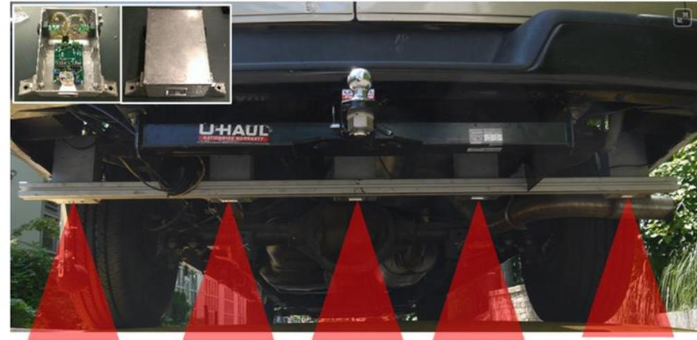
VOTERS millimeter-wave radar systems mounted underneath the van is capable of detecting metal objects on the road and is used to identify the manholes.
