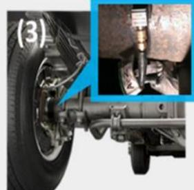
(3) Rear axle accelerometer
