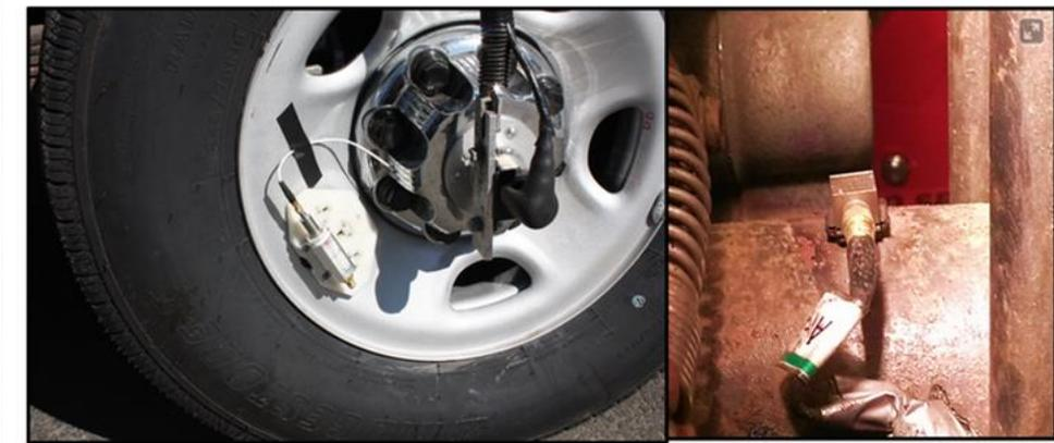
Through VOTERS Dynamic Tire Pressure Sensor and an axle-accelerometer, International Roughness Index (IRI) has been quantified. IRI has been used worldwide for evaluating and managing highways since the early 1980s. IRI is highly related to the ride quality or comfort experienced by a driver.
