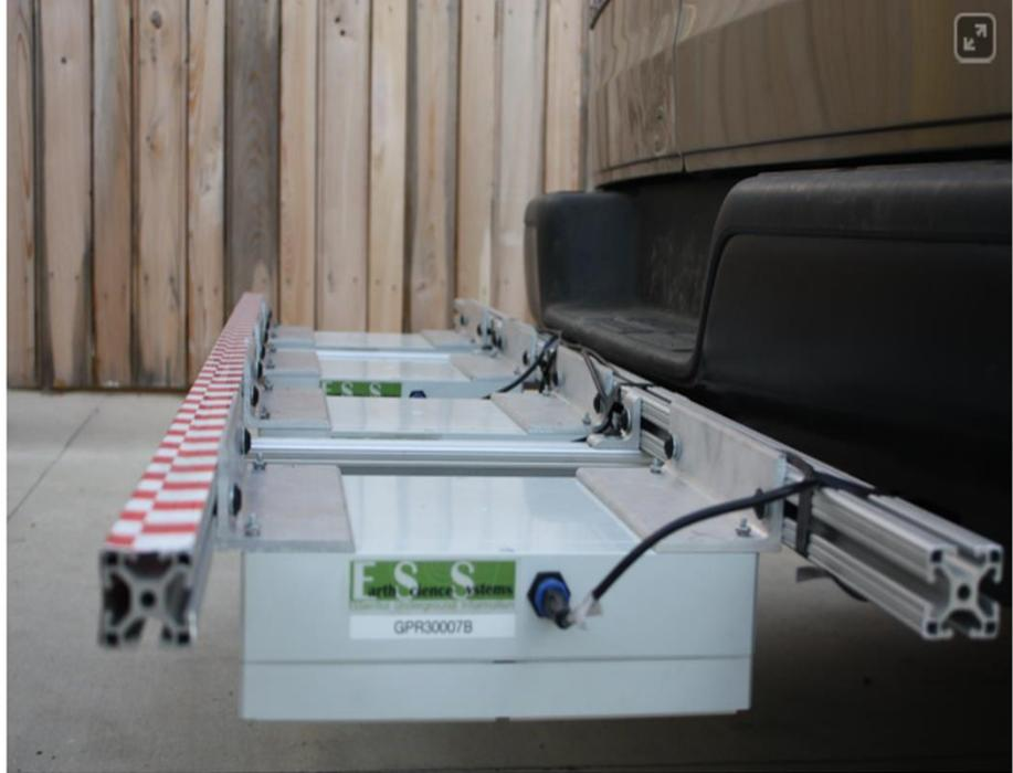
VOTERS can provide Pavement Layer profiling with air-coupled GPR in addition to dielectric constant, providing more insight into condition of pavements to help with a better maintenance planning.
