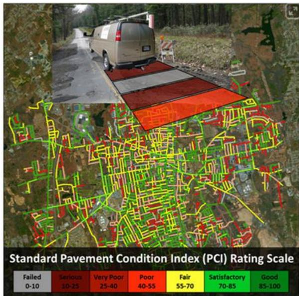
Pavement Condition Index (PCI) is the main measure used in the US to assess road conditions. PCI is between 0-100 (100 for a good condition and 0 for a failed condition).
