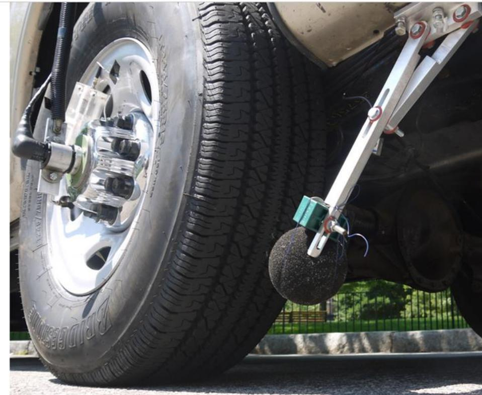
Macrotexture is highly correlated to tire/road friction hence related to the severity of the sound generated by tire-pavement interaction. MTD shows severity of segregation and raveling, two dominant types of pavement distress.
