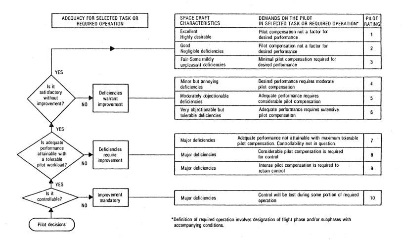
Figure 8: Cooper-Harper subjective rating scale
