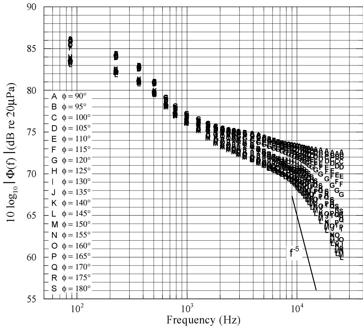
**Figure 108.** Power spectra of surface pressure fluctuations at  $\alpha = 10^\circ$ ,  $x/L = 0.600$ .
