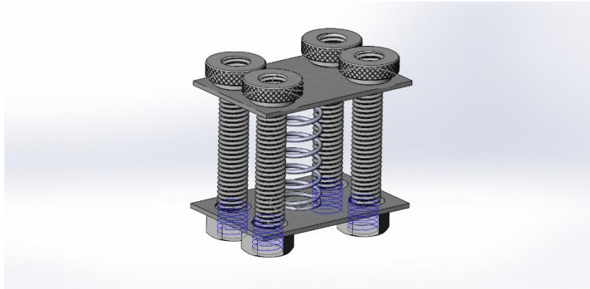
Figure 4-2 Three-dimensional diagram of the system used to apply compression to the sandwich structures.
