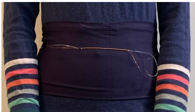
Figure 5-6 Picture of Respiration Sensor A double coil fiber was stitched onto a running storage belt.
