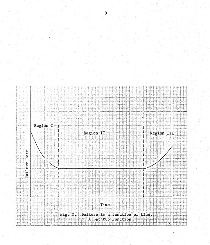
If structural components of a mechanism are mass produced, the strength at failure Y of each single component may be considered a random variable. The component is installed in an assembly and exposed to a stress which reaches its maximum value X, again a random variable. If Y < X, then the component will fail in use.
