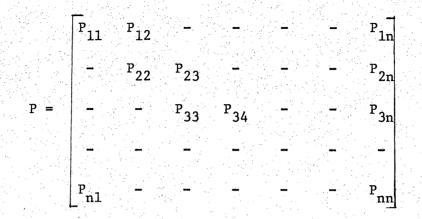
Deterioration in one time period is not sufficient for the component to change through two states. In any one time period the component can exist in any one of the  $S_1, S_2 \dots S_n$  states. This system can be represented by a Markov Process.
