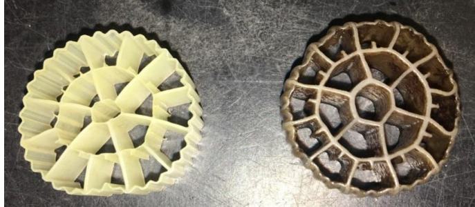
Figure 13: Virgin carrier (left) versus preliminary biofilm carrier (right).
